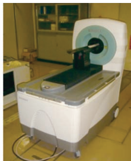
Fig.4-25 Chemical structure of ^{76}\text{Br} -MBBG (left) and photo of a small-animal PET (right)
