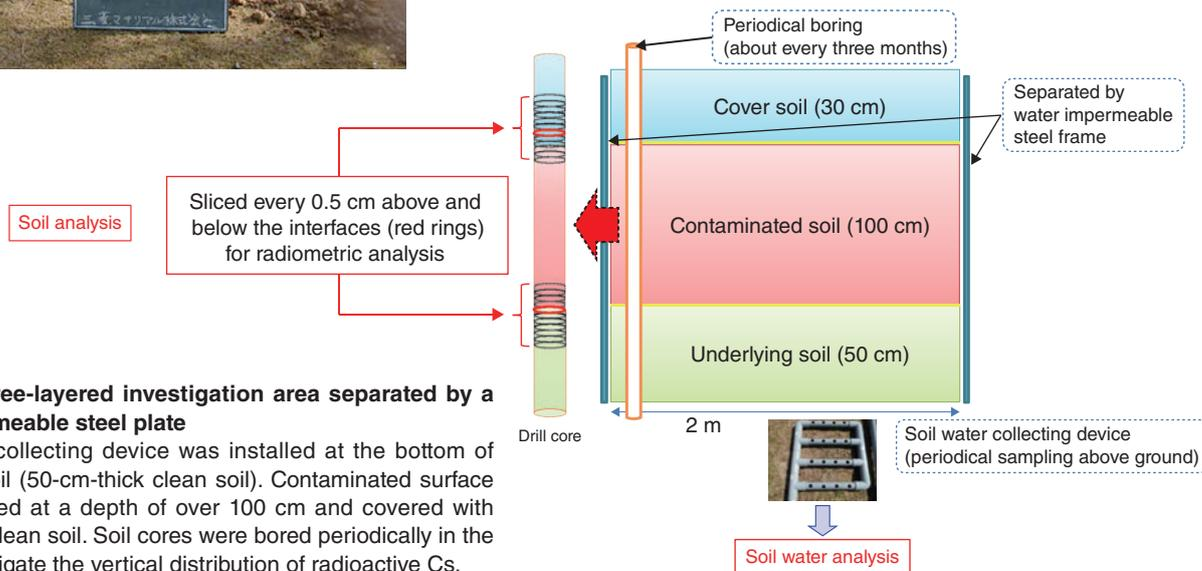
**Fig.1-39 Three-layered investigation area separated by a water-impermeable steel plate**
