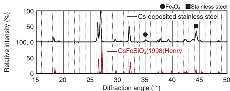
**Fig.1-14 XRD patterns of Cs-chemisorbed stainless steel and CsFeSi<sub>4</sub>**
