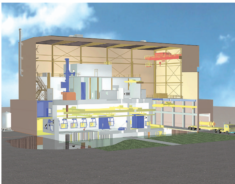
Fig. 8: Conceptual sketch of Semi-Full Scale Post-Irradiation Examination Facility for Monju
