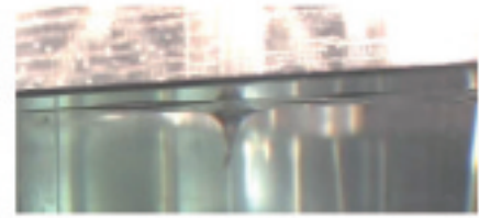
(1) Flow visualization of gas entrainment due to dimple vortex in the water experiment
