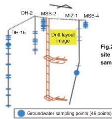
Fig.2-16 Bird's-eye view of MIU construction site and borehole location, and groundwater sampling point in each borehole.
