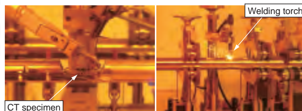
Fig.12-12 Photographs of assembling work of the IASCC test capsule in hot cell
