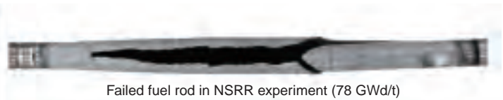
Fig.5-5 Pulse irradiation experiment at NSRR
