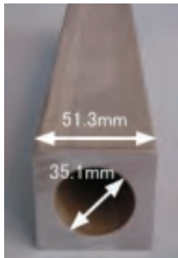
Fig.3-25 Photo of full size CS circle-in-square conduit made of improved JK2 In inspection, ITER requirement for size precision was satisfied. After insertion of superconducting cable into conduit, the conduit is compacted to 49 mm square.
