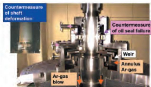
Fig.1-31 Countermeasures of mechanical sodium pump
