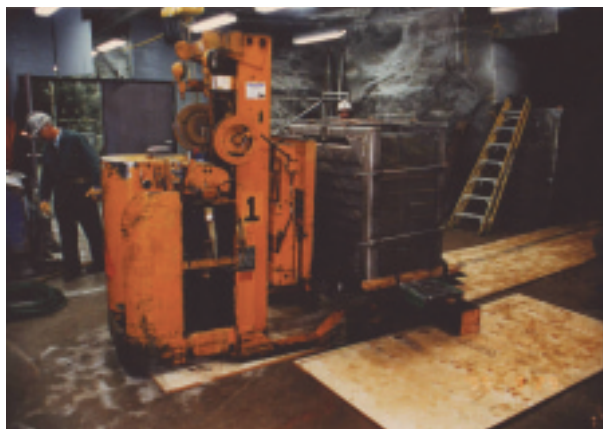
Fig.5-17 Forklift transporting granite block containing natural fracture, quarried at a depth of 240 m
