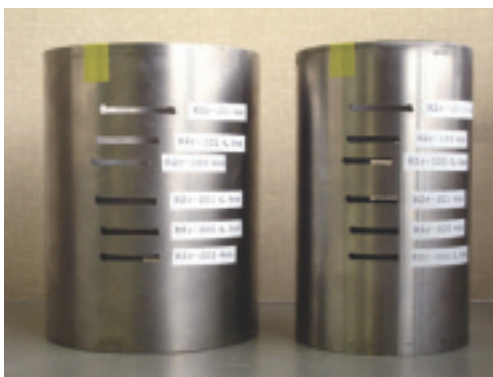
Fig.9-3 Specimen used in the experiment (The tubes were arranged coaxially and cut from inside simultaneously)
