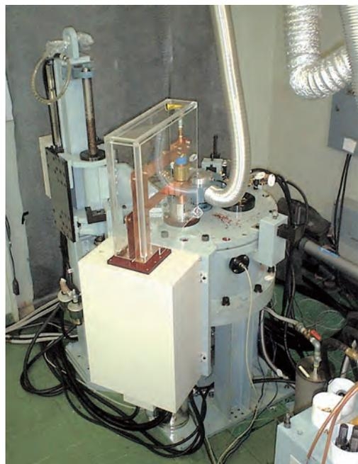
**Fig.6-6 Mega-gravity generator (JAEA)**
