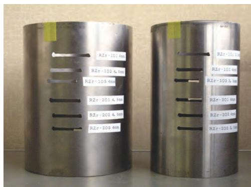
Fig.9-3 Specimen used in the experiment (The tubes were arranged coaxially and cut from inside simultaneously)
