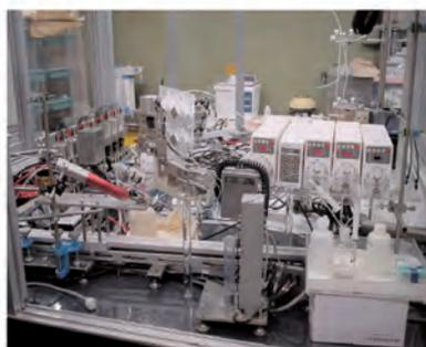
Automated rapid ion-exchange apparatus AIDA for the study of liquid-chromatographic behavior of superheavy elements.
