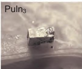
Single crystal growth of a plutonium compound  $PuIn_3$  and observation of its Fermi surface.
