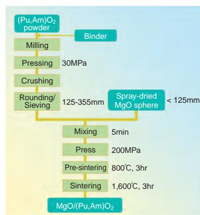
**Fig.1-8 Fabrication process of macro-dispersed type fuel**
