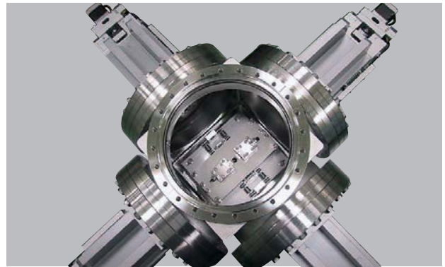
Divergence defining slit for formation of a heavy ion micro beam of a several hundred MeV class
