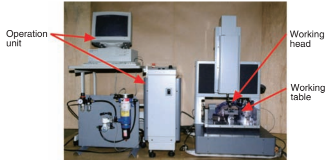
(b) Processing machine By using a manipulator for remote-handling, it is easy to fix the specimen onto the remote-controlled NC lathe. This machine warrants the high accuracy of processing, the same as the out of the hot cell processing.
