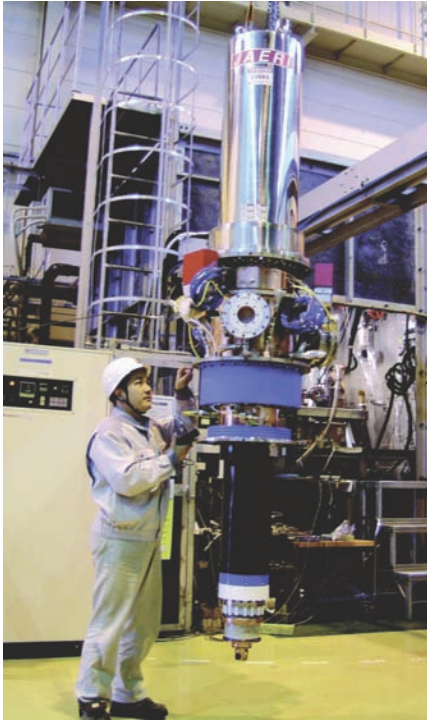
Fig.3-10 The plasma heating device “gyrotron” for ITER
