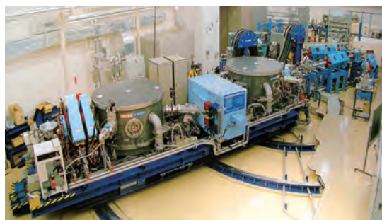
Recoil mass separator for experimental research on fusion reaction mechanisms to produce super-heavy elements by bombarding deformed nuclei with heavy-ion beams from JAEA tandem-booster accelerator.
