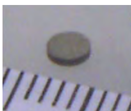
Fig.7-7 Sintered AmN disk sample
