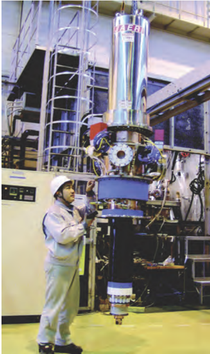
Fig.3-10 The plasma heating device “gyrotron” for ITER
