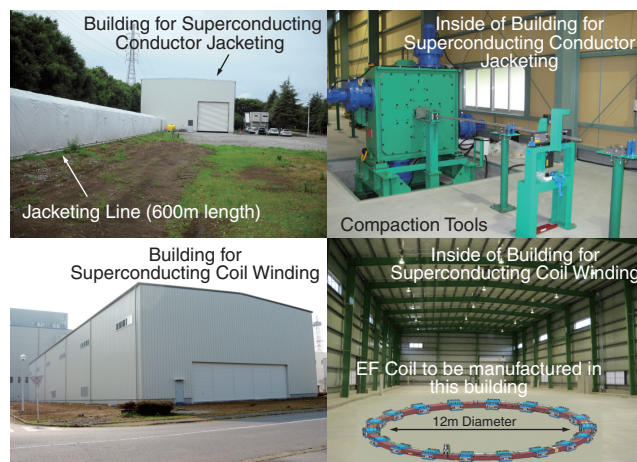
Superconducting Strands Jacketing Building and Superconductor Winding Building and their interiors
