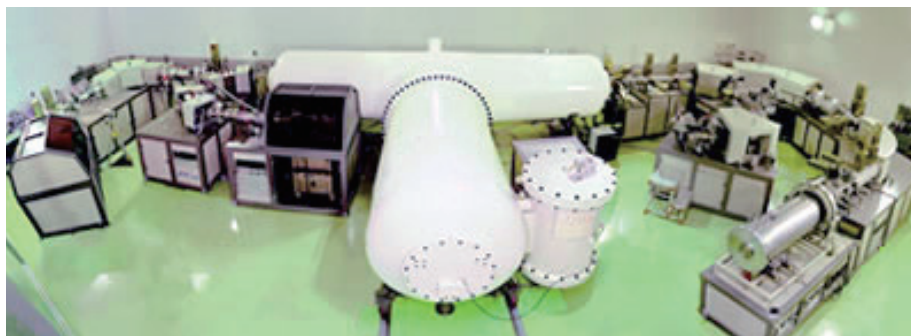
Fig.14-29 Accelerator Mass Spectrometer (AMS) at Aomori Research & Development Center This AMS can measure ^{129}\text{I} in environmental samples which could not be measured previously.
