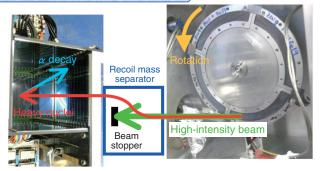
Physical and chemical properties of unknown heavy nuclei are investigated. Nuclei are synthesized in fusion reactions when a rotating target (right) is bombarded by high-intensity heavy-ion beams, separated from the incident beam by a recoil mass separator, and then implanted into a silicon-strip detector (left) which observes the  $\alpha\text{-}\text{decay}$  chain.
