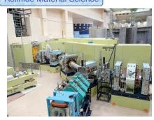
$\mu \text{SR}$  spectroscopy system installed at J-PARC Muon Facility. The system is able to detect the extremely small magnetic field to elucidate physical properties of materials, behavior of hydrogen atoms, etc., in substances.
