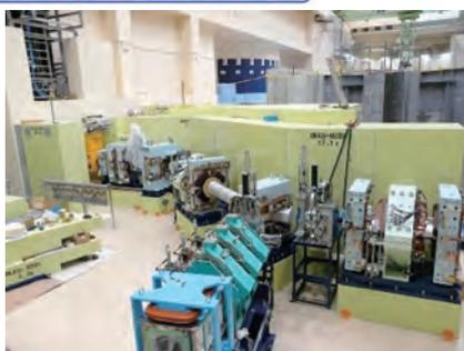
$\mu$ SR spectroscopy system installed at J-PARC Muon Facility. The system is able to detect the extremely small magnetic field to elucidate physical properties of materials, behavior of hydrogen atoms, etc., in substances.
