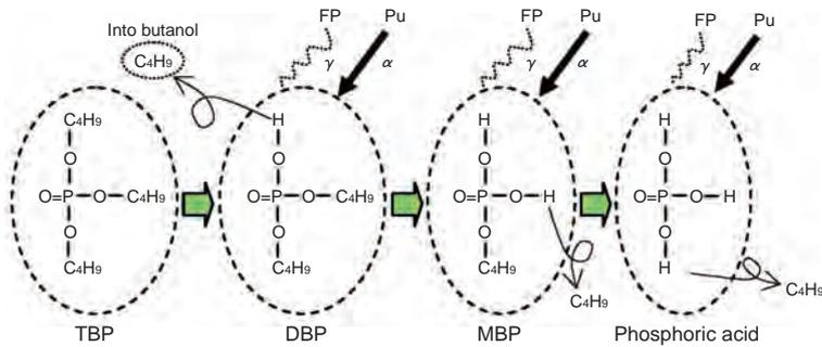
**Fig.8-3 Solvent degradation**
