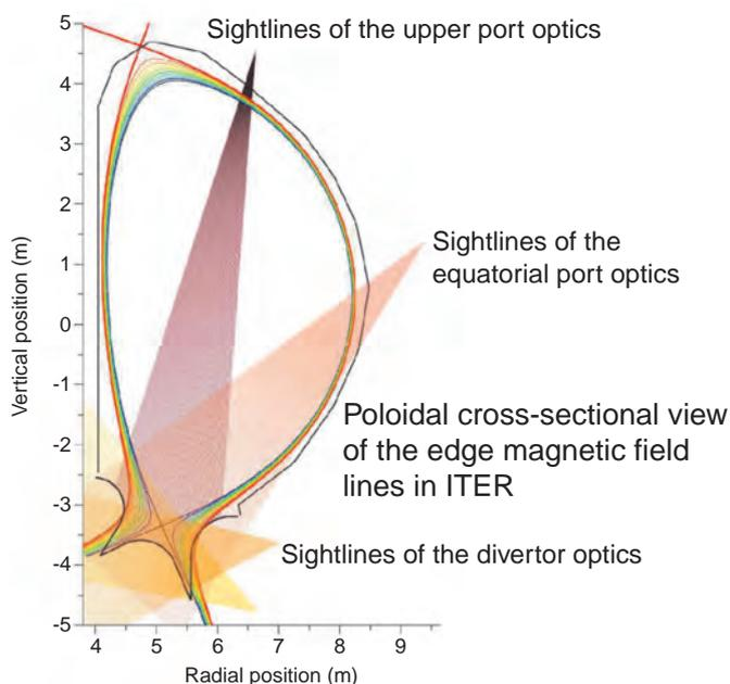
**Fig.3-16 Sightlines of impurity influx monitor (divertor)**
