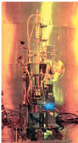
**Fig.7-9 Appearance of corrosion testing apparatus**
