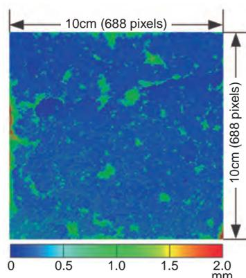
**Fig.2-6 Example of fracture aperture measurement**
