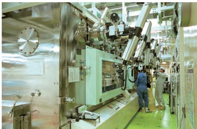
**Fig.7-12 Module for TRU high temperature chemistry**
