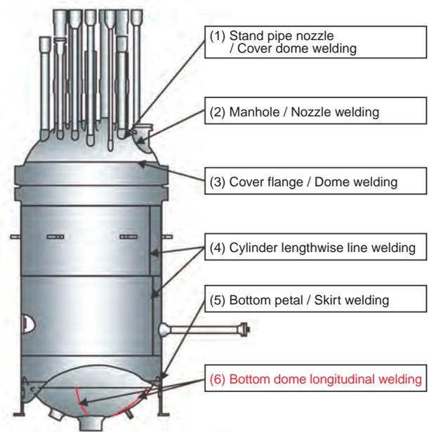
**Fig.14-21 Main welding lines of the RPV of HTTR**
