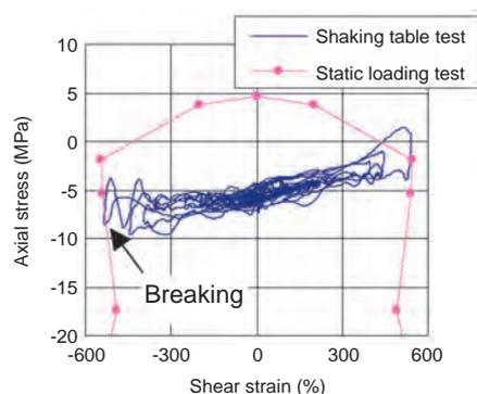
**Fig.1-21 Breaking strain of laminated rubber bearing**
