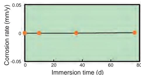
**Fig.14-19 Relationship between immersion time and corrosion rate of SS304**
