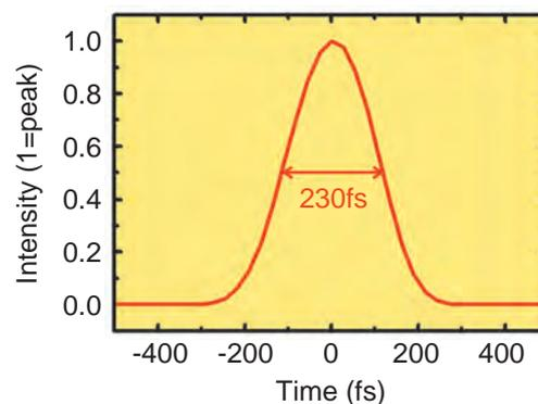
**Fig.11-6 Recompressed pulse waveform**
