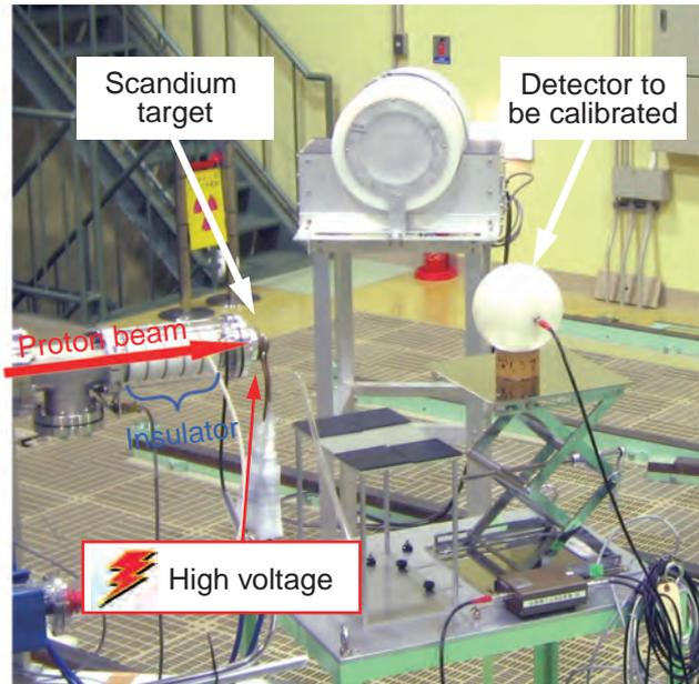
**Fig.14-4 Setup in the mono-energetic neutron calibration fields**
