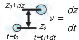
**Fig.1-28 Method for estimation of bubble surfacing velocity**
