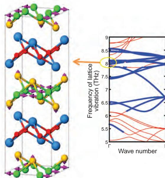
**Fig.12-8 Visualization of the lattice vibration in the iron-based superconductor LaFeAsO and its dispersions**
