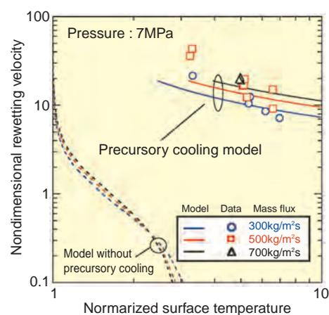
**Fig.5-10 Comparison of measured and calculated rewetting velocities**
