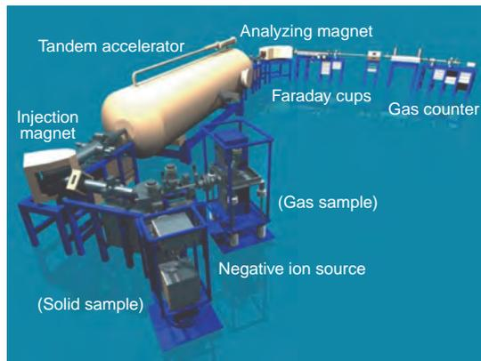
**Fig.2-12 Outline of pelletron dating instrument**
