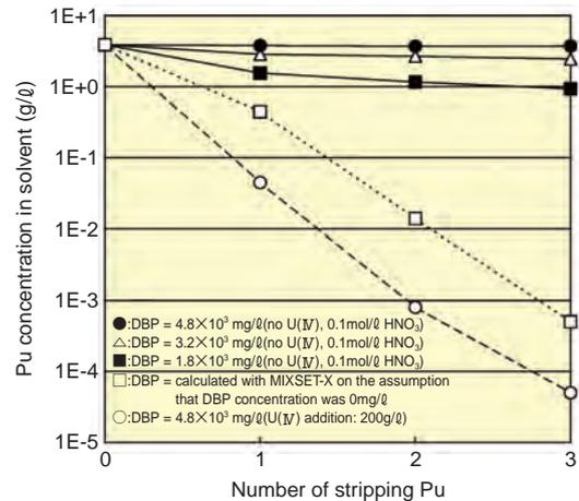
**Fig.8-4 Pu concentration after stripping Pu in solvent**
