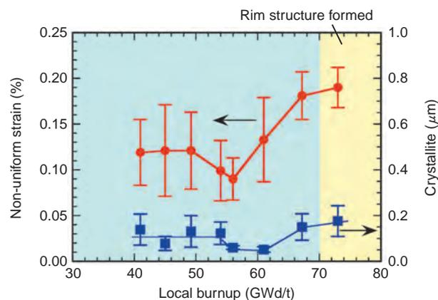
**Fig.5-7 Local burnup dependence of non-uniform strain and crystallite size in the irradiated fuel pellets**
