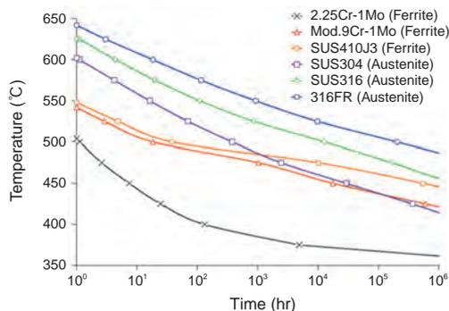
Fig.1-11 Proposed negligible creep curves for each material
