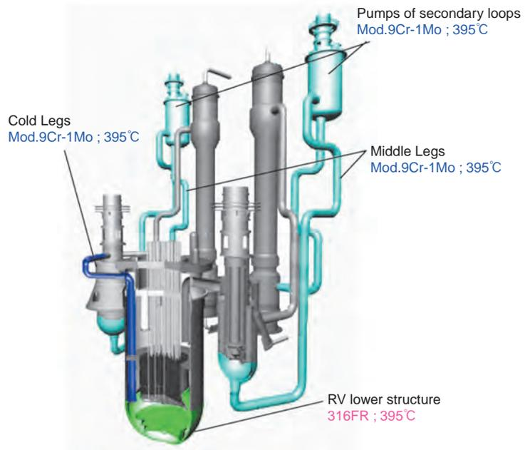
Fig.1-12 Components with negligible creep effect in design
