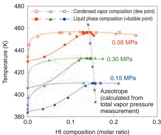
**Fig.7-21 VLE data of HI+H<sub>2</sub>O mixture**
