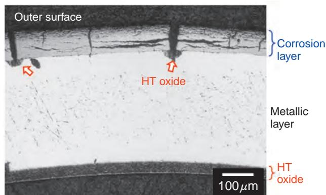
**Fig.5-5 Radial cross section of the irradiated ZIRLO cladding after high-temperature oxidation test**
