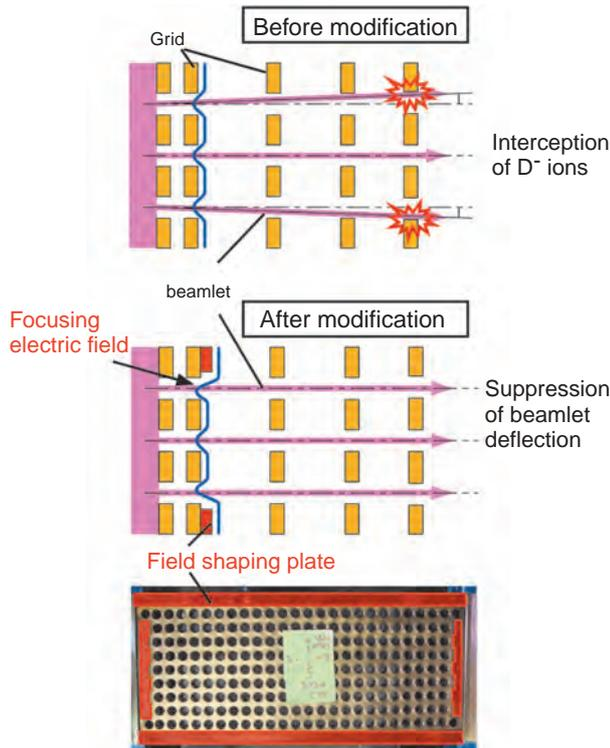
**Fig.3-9 Schematic diagram of beam trajectories before and after modification**
