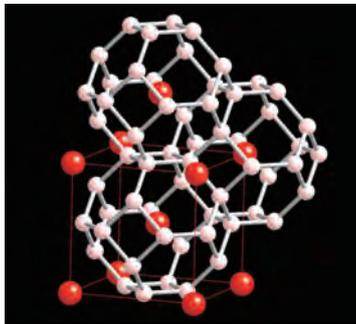
Fig.14-14 Positions of vacancies (white balls) where hydrogen can enter in a body-centered cubic lattice (red balls)
