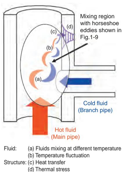
**Fig.1-7 Thermal striping in a T-junction piping system**
