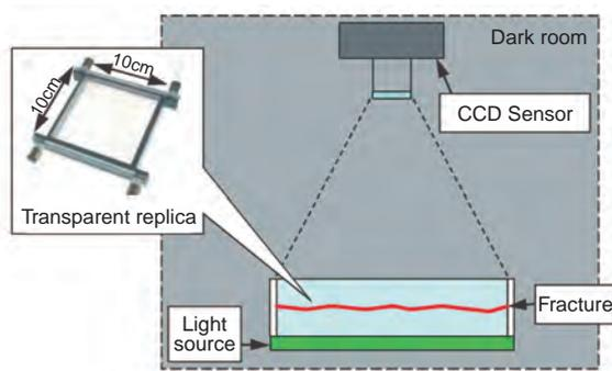
**Fig.2-5 Concept of optical measurement of a fracture**
