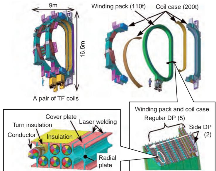
Fig.3-14 Configuration of TF coil
