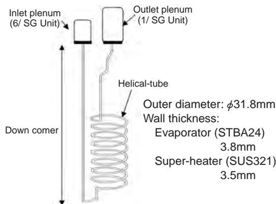
Fig.14-2 Steam Generator Tube (1 Tube)
