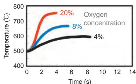
**Fig.1-17 Internal temperature of the liquid droplet**
