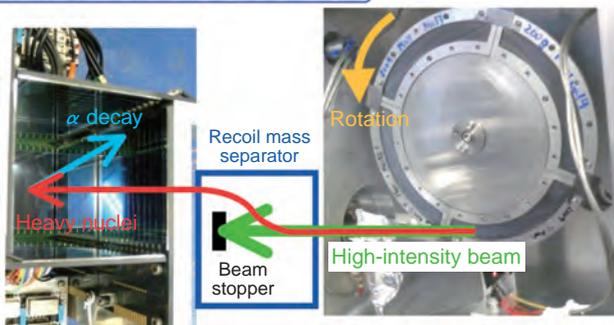
Physical and chemical properties of unknown heavy nuclei are investigated. Nuclei are synthesized in fusion reactions when a rotating target (right) is bombarded by high-intensity heavy-ion beams, separated from the incident beam by a recoil mass separator, and then implanted into a silicon-strip detector (left) which observes the  $\alpha$ -decay chain.
