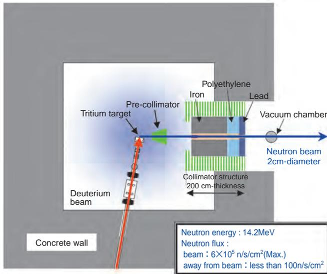
**Fig.3-23 Schematic view of the charged-particle double-differential cross-section measurement system at the FNS facility**
