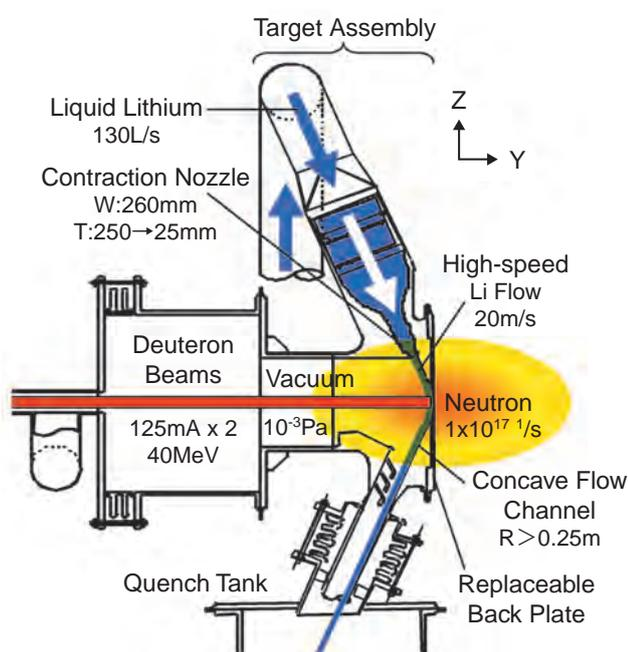
**Fig.3-25 Concept of IFMIF liquid lithium (Li) target**
