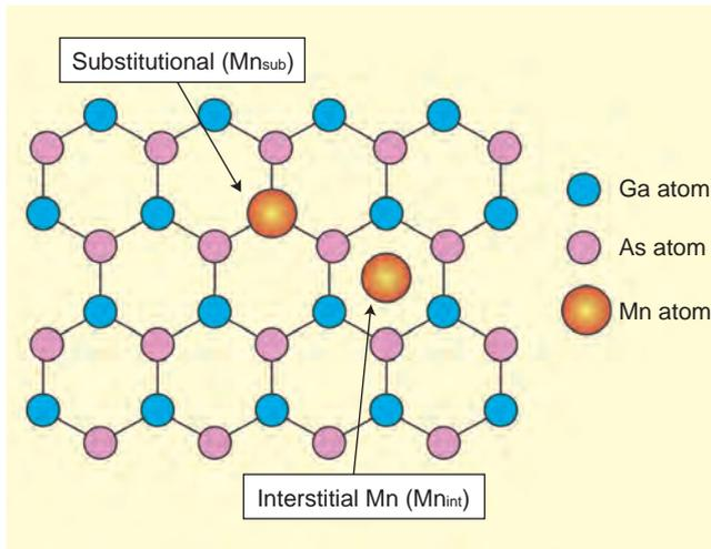
**Fig.4-4 Schematic view of Ga<sub>1-x</sub>Mn<sub>x</sub>As (111) surface**
