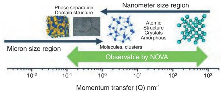
Fig.14-13 Momentum transfer ( $Q$ ) range observed by NOVA
