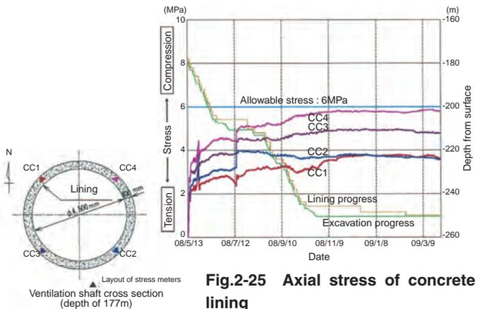
**Fig.2-25 Axial stress of concrete lining**
