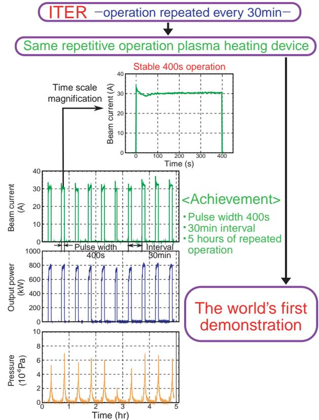
**Fig.3-20 Repetitive gyrotron operation**
