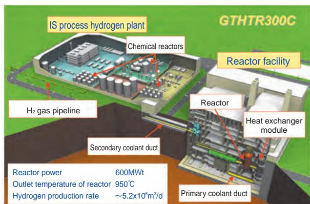
**Fig.7-22** Bird's eye view of GTHTR300C
