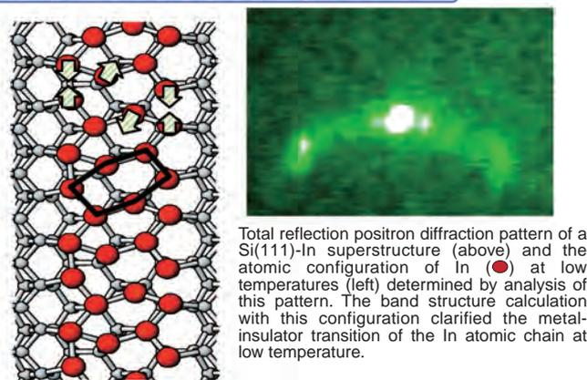
Total reflection positron diffraction pattern of a Si(111)-In superstructure (above) and the atomic configuration of In (●) at low temperatures (left) determined by analysis of this pattern. The band structure calculation with this configuration clarified the metal-insulator transition of the In atomic chain at low temperature.
