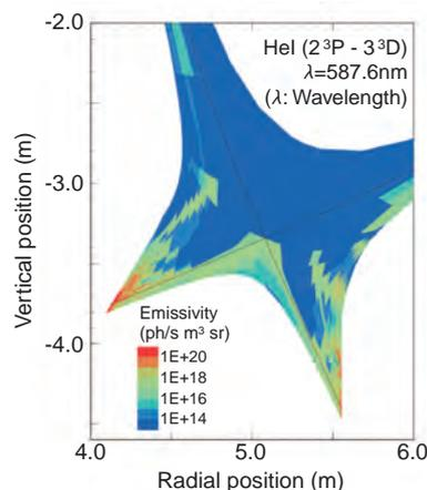
**Fig.3-18 Helium atom spectral line emissivity of divertor (Hel:wavelength 587.6nm)**
