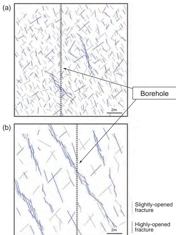
**Fig.2-19 Conceptual model for connectivity of fractures**
