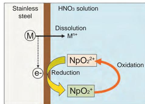
**Fig.7-11 Schematic illustration of corrosion mechanism in HNO<sub>3</sub> solution with neptunium**
