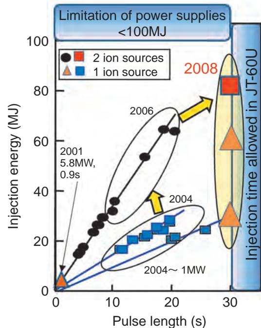
**Fig.3-10 Injection energy achieved in negative-ion-based NBI (N-NBI) in JT-60U**
