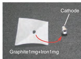
**Fig.2-13 Preparation of a measuring sample**
