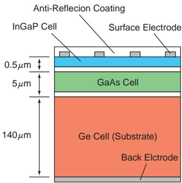
**Fig.4-8 A cross-sectional diagram of InGaP/GaAs/Ge triple-junction solar cell**
