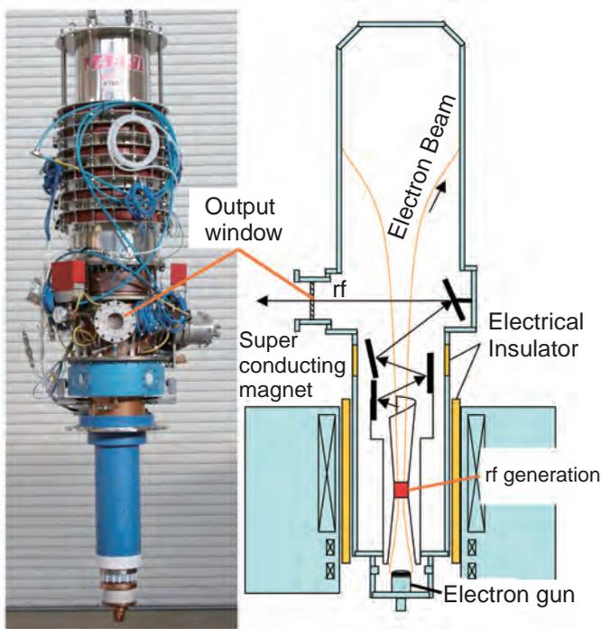
**Fig.3-19 Millimeter wave plasma heating device; Gyrotron**
