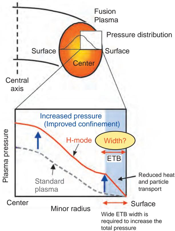
**Fig.3-5 Spatial profile of plasma pressure in H-mode**
