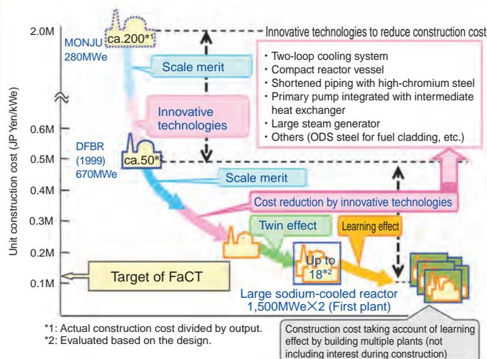
**Fig.1-3 Approaches to reduce construction cost**
