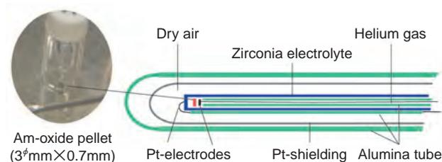
**Fig.7-13 Electrochemical cell with a zirconia electrolyte**
