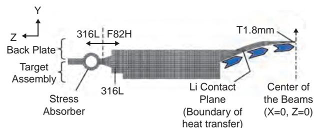
**Fig.3-26 Thermal stress analysis model**
