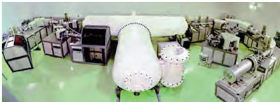
**Fig.14-29 Accelerator Mass Spectrometer (AMS) at Aomori Research & Development Center**
