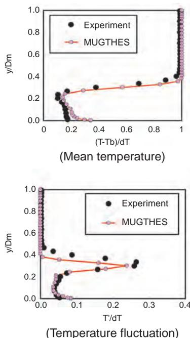
**Fig.1-8 Radial profiles of fluid temperature**
