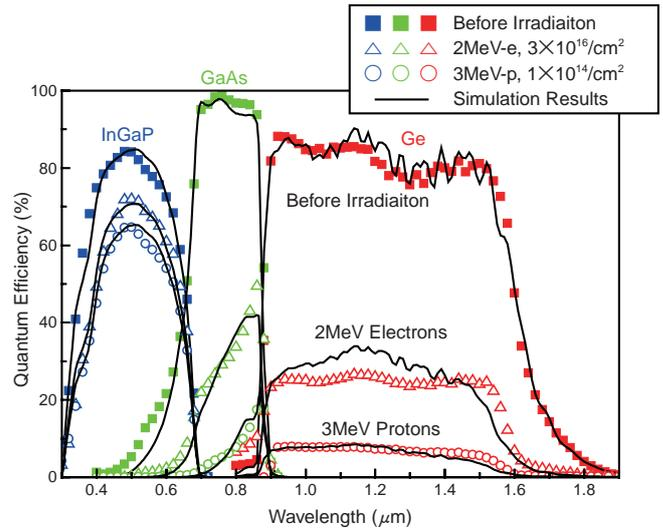
**Fig.4-9 Quantum efficiencies of 3J cells irradiated with 3MeV protons or 2MeV electrons**
