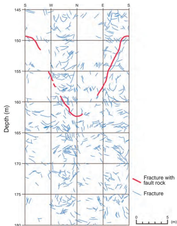
**Fig.2-20 Observed fractures in shaft wall**
