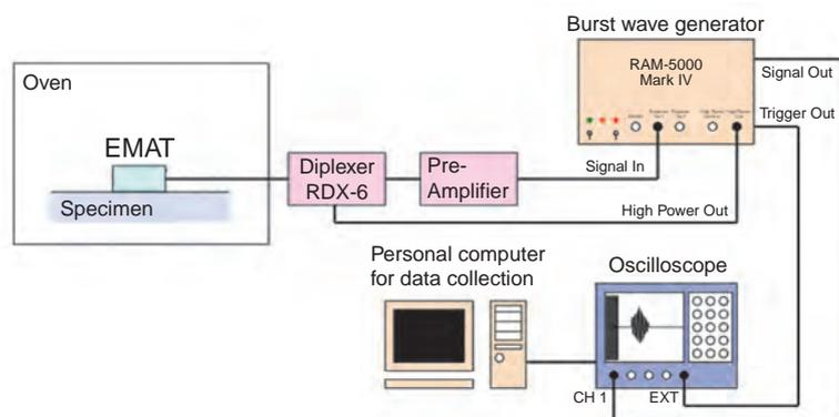
Fig.1-13 Measurement system
