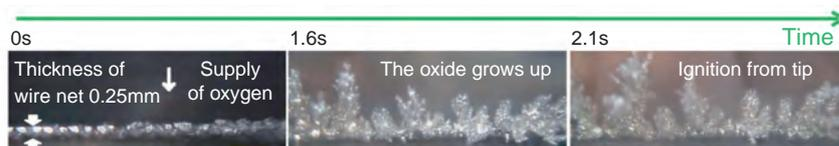
**Fig.1-18 Growth of the columnar oxides**
