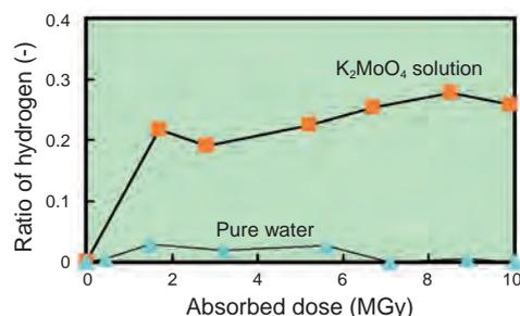
**Fig.14-18 Relationship between absorbed dose of  $\text{K}_2\text{MoO}_4$  solution and ratio of hydrogen in generated gas**
