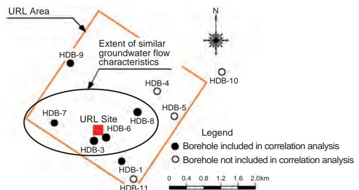
Fig.2-23 Image of area with similar groundwater flow characteristics (400m in depth)
