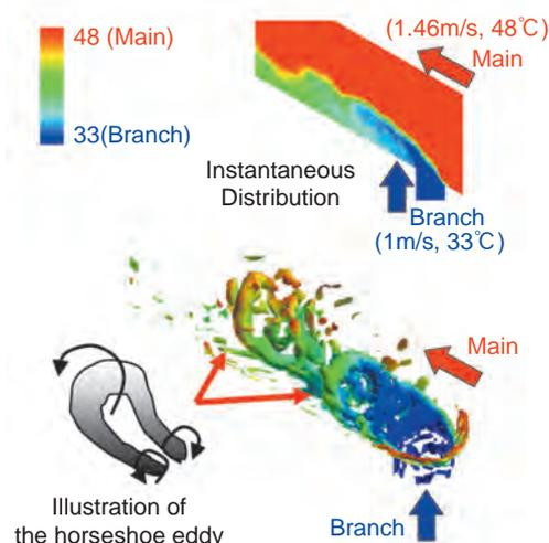
**Fig.1-9 Horseshoe eddies showing Iso-Surfaces of rotating flow strength**
