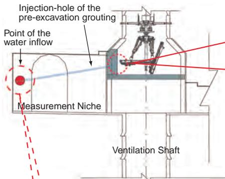
**Fig.14-24 GL-200m Measurement Niche off Ventilation Shaft**
