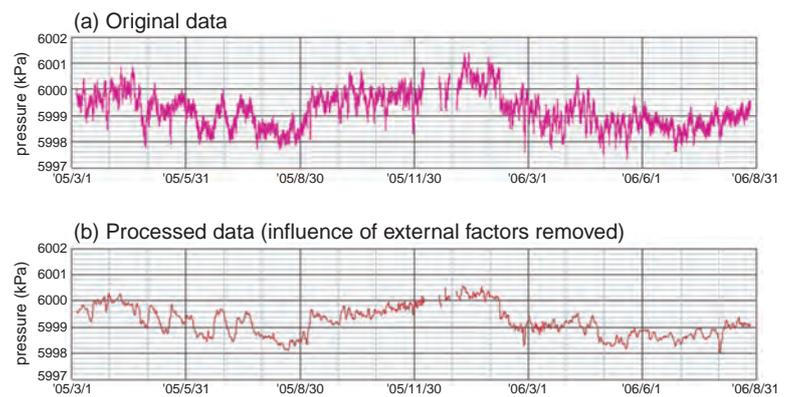
Fig.2-22 BAYTAP-G (Tamura, Y. et al., *Geophysical Journal International* vol.104, 1991), Example of groundwater pressure monitoring data (HDB-6: 585-620m in depth)
