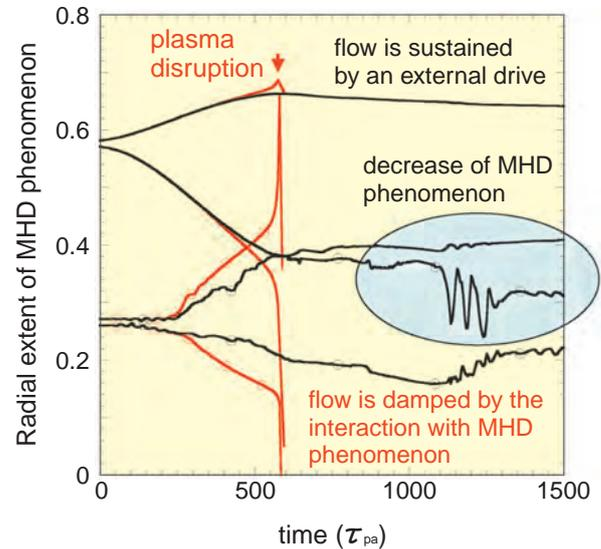
**Fig.3-8 Avoidance of the low pressure disruption by the plasma flow in the advanced plasma discharge**
