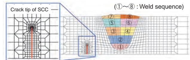
**Fig.5-12 2D FEM model for welding simulation and SCC**
