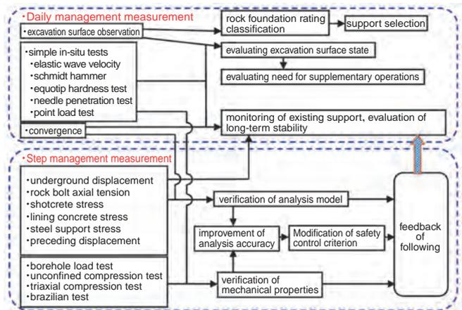
**Fig.2-24 Observational construction flow**
