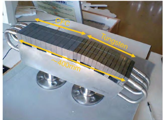
**Fig.3-22 ITER divertor prototype**
