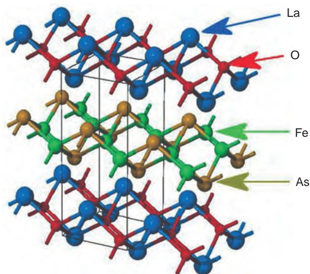
**Fig.12-7 Crystal structure of the first iron-based superconductor LaFeAsO**
