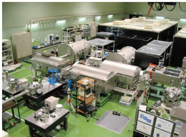
Plasma X-ray Laser apparatus
