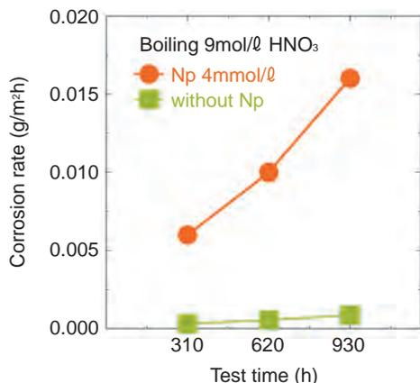
**Fig.7-10 Corrosion rate of stainless steel in boiling HNO<sub>3</sub> solution at 70°C**
