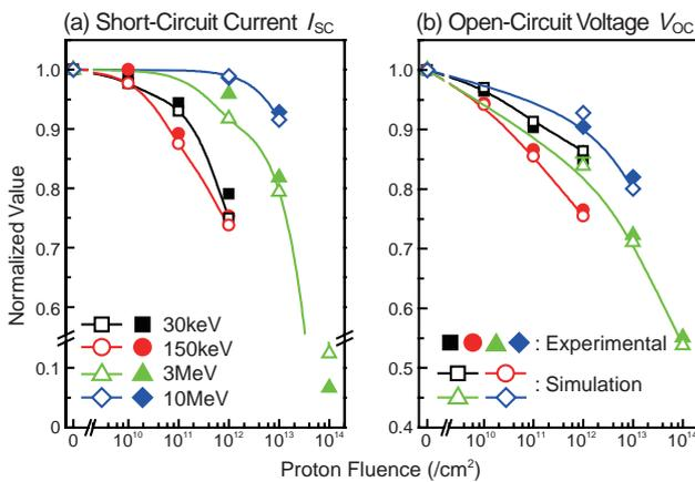
**Fig.4-10 Curves of (a)  $I_{sc}$  and (b)  $V_{oc}$  for 3J cells during four levels of proton irradiation**
