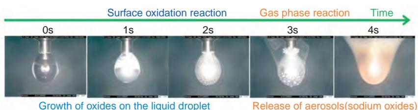
**Fig.1-16 Event transition of sodium combustion 20%O<sub>2</sub>**
