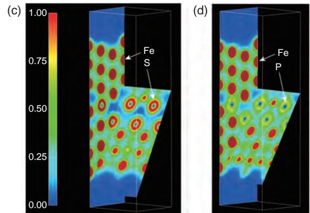
**Fig.12-3 Electron distribution map at the grain boundary when sulfur (S) or phosphorous (P) atoms are segregated (c) S. (d) P.**
