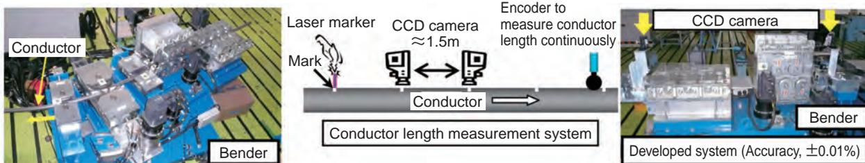
Fig.3-15 High accuracy winding system
