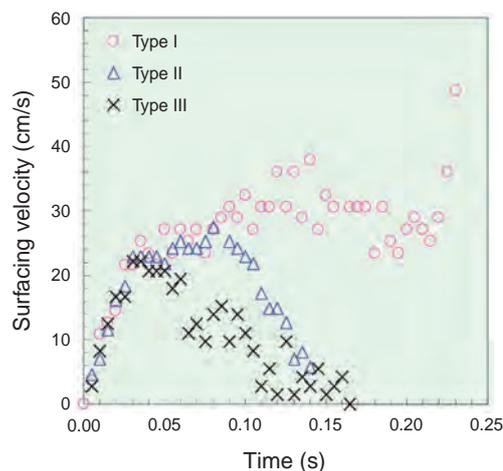
**Fig.1-29 Surfacing velocity of bubble (Different vessels)**
