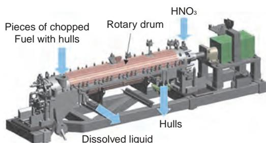
**Fig.1-22 Rotary Drum Type Continuous Dissolver**
