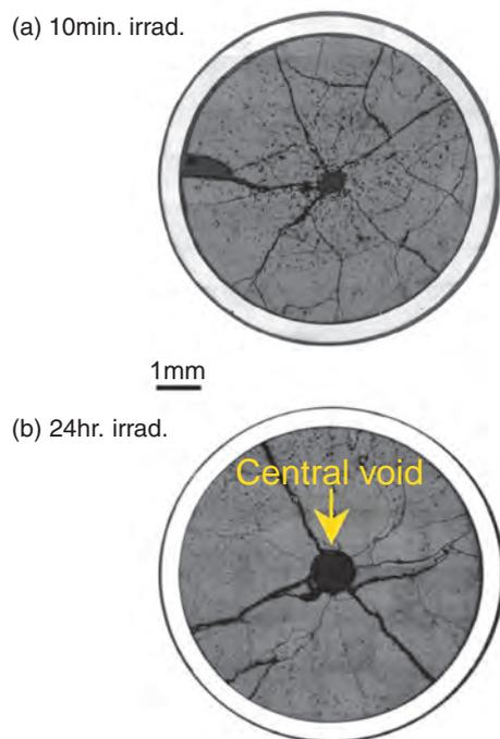
**Fig.1-5 Ceromography of irradiated 5% Am-MOX fuel**
