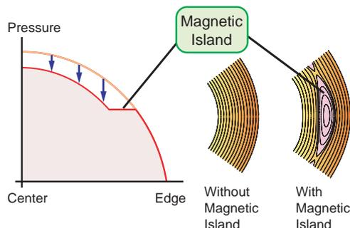
**Fig.3-2 Pressure profiles with and without magnetic island**
