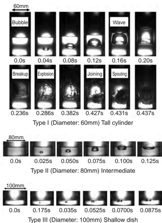
**Fig.1-26 Observation of spouting caused by MH**
