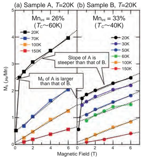
**Fig.4-5 Magnetic dependence of the spin moment ( $M_s$ ) of Ga<sub>1-x</sub>Mn<sub>x</sub>As at  $T = 20\text{K}$**
