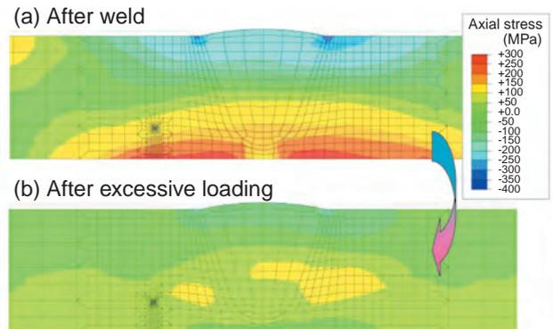
**Fig.5-13 Effect of earthquake on weld residual stress**
