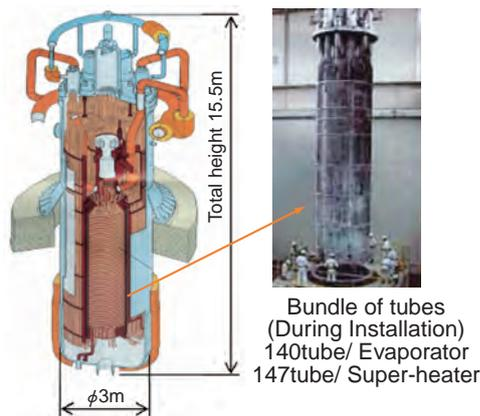
Fig.14-1 Steam Generator (Evaporator)
