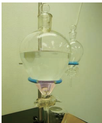
Fig.14-33 Iodine extraction from seawater samples
