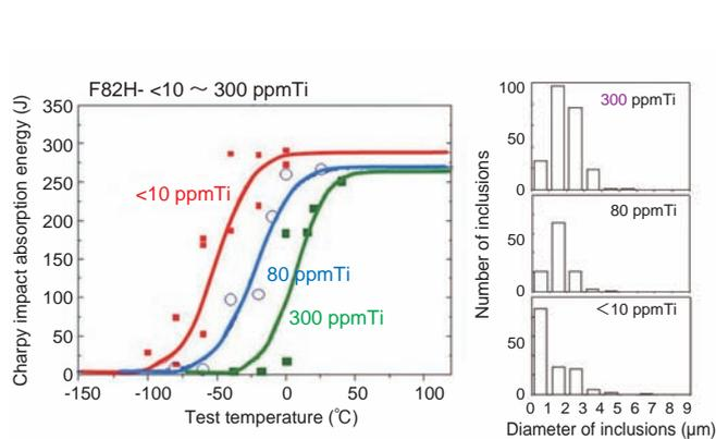
**Fig.3-27 The impact of Ti contamination level in F82H**
