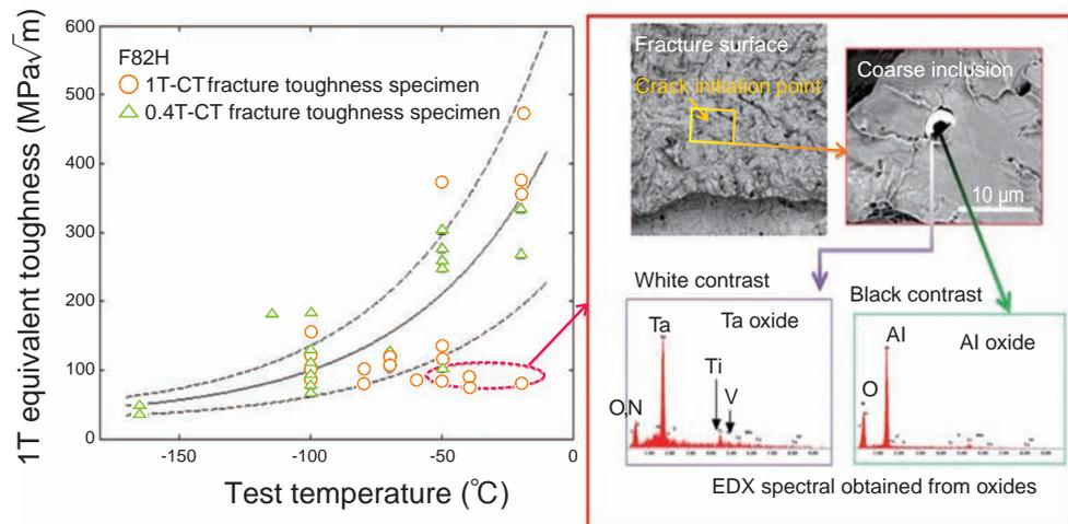
**Fig.3-26 The influence of inclusions on the toughness of F82H**
