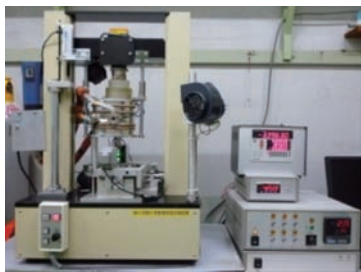
Fig.3-30 We developed test equipment (left) of fracture toughness for small size specimens (right)
