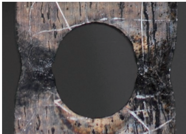
Fig.8-11 Deformation behavior of an intensely irradiated structure with a discontinuity
