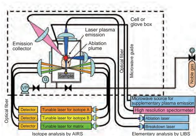
**Fig.13-2 Concept of MOX sample verification system for FNFC using LIBS/AIRS**
