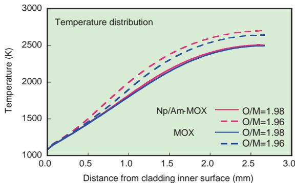
**Fig.1-22 Radial temperature distribution in the pellet**
