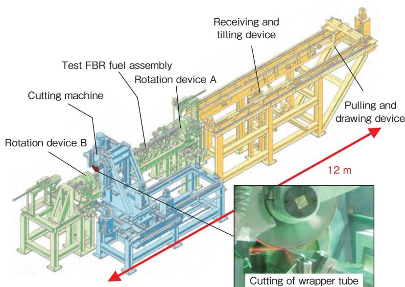
**Fig.1-12 Engineering-scale test machine for disassembly operation**
