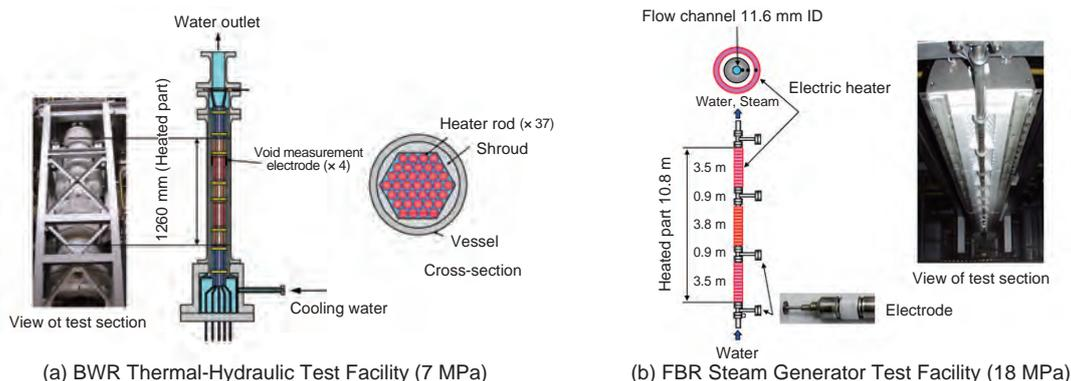
**Fig.14-4 Test facilities applied to the capacitance void measurement method**
