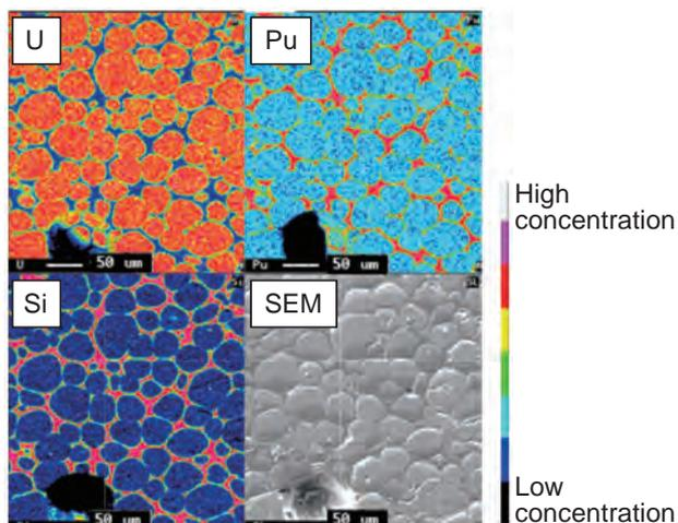
**Fig.1-23 Element mapping images of MOX-6.9 wt%SiO<sub>2</sub> analyzed by EPMA**
