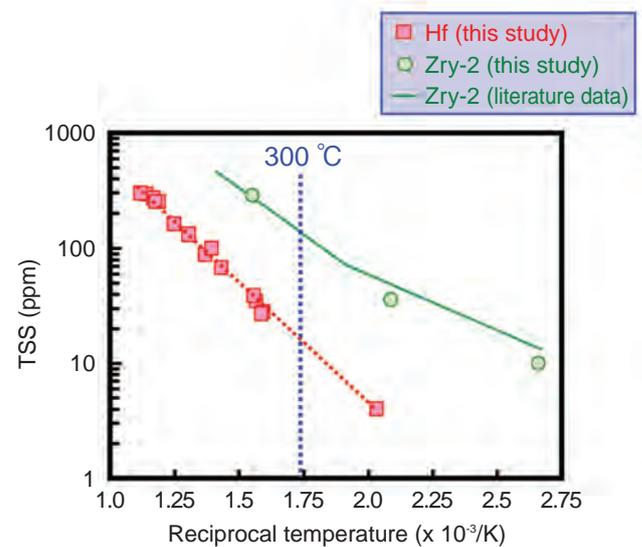
**Fig.6-7 Temperature dependence of terminal solid solubility of hydrogen (TSS): a comparison between Hf and zircaloy-2 (Zry-2)**
