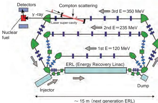
**Fig.13-3 Concept of Pu NDA system for spent fuel using NRF with interrogation of LCS  $\gamma$ -rays**
