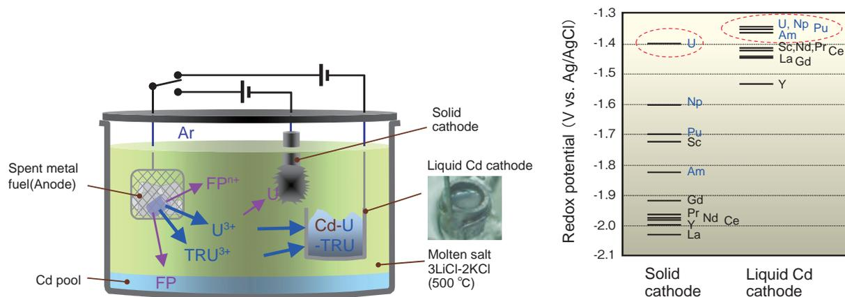
**Fig.1-25 Concept of the electro-refining process and standard redox potential of TRU and rare earth elements**
