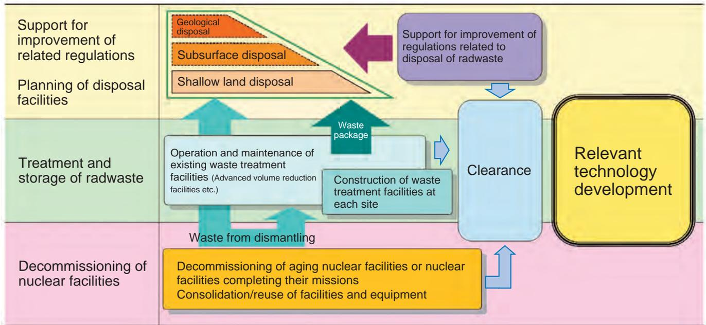
Fig.11-1 Outline of measures for decommissioning and radwaste treatment & disposal
