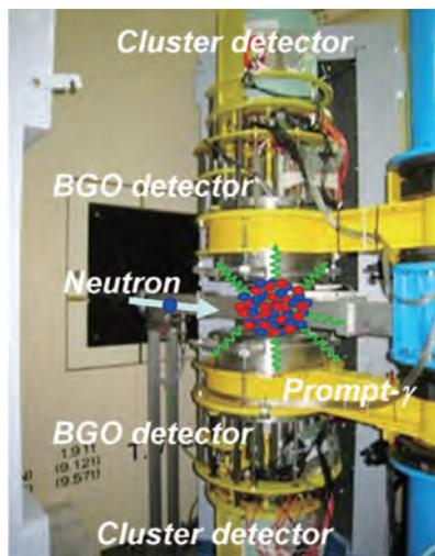
**Fig.8-6 A photo of the 4π Ge spectrometer**
