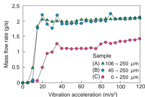
**Fig.1-19 Flowability profiles of ZrO<sub>2</sub> smaller than 250 μm**
