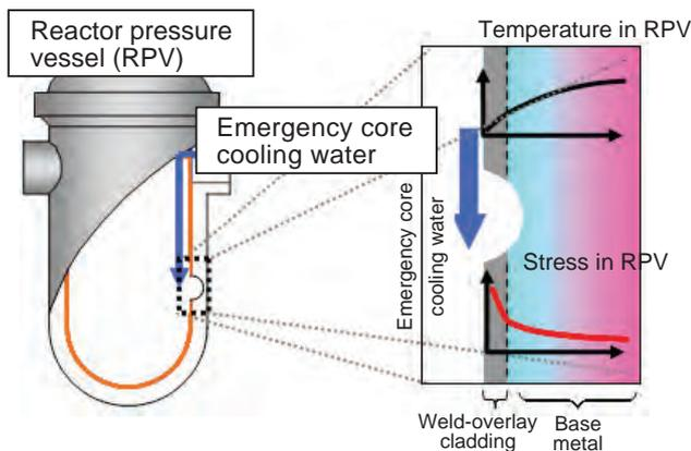
**Fig.6-10 RPV pressurized thermal shock event of RPV**
