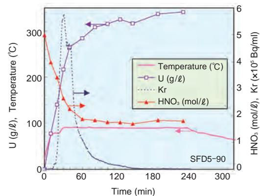
Fig.8-2 Changes in temperature and composition of working solution, and release behavior of Kr during MOX dissolution
