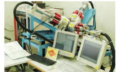
**Fig.11-7 Multi parameter coincidence spectrometer**
