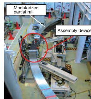
**Fig.3-8 Demonstration for assembly of modularized partial rail**
