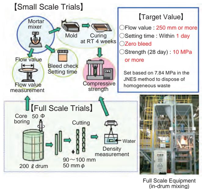
**Fig.10-5 Diagram of cement based encapsulation trials**
