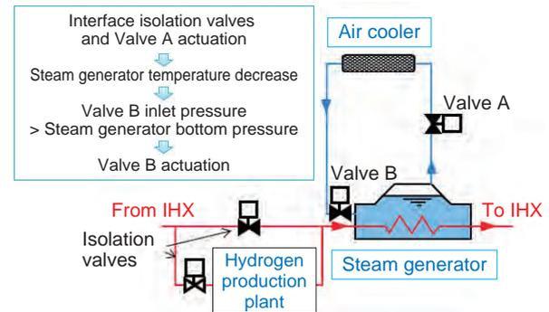
**Fig.9-6 Sequence control for mitigation of load variation**
