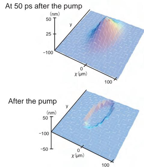
**Fig.4-9 Retrieved surface profile from the interferogram**
