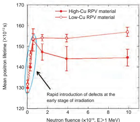
**Fig.6-8 Mean positron lifetimes as a function of neutron fluence**
