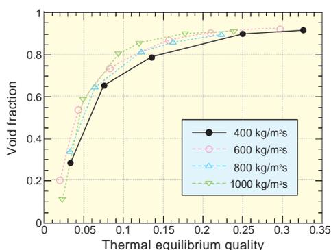
**Fig.14-5 Result of void fraction measurement in BWR thermal hydraulic testing**
