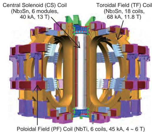
**Fig.3-2 ITER superconducting magnet system**
