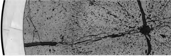
**Fig.1-20 Cross-sectional microstructure of Np/Am-MOX pellet irradiated at 430 W/cm for 10 min**
