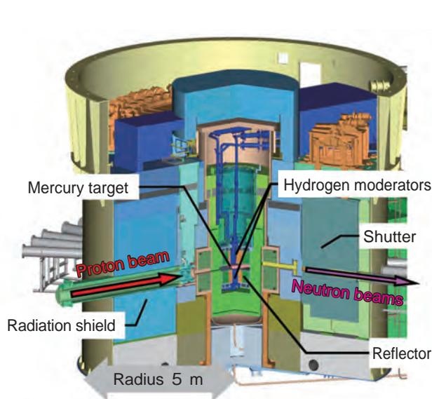
**Fig.14-12 1 MW pulsed neutron source at J-PARC**
