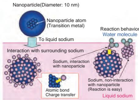
**Fig.1-29 The concept of sodium with suspended nanoparticles**
