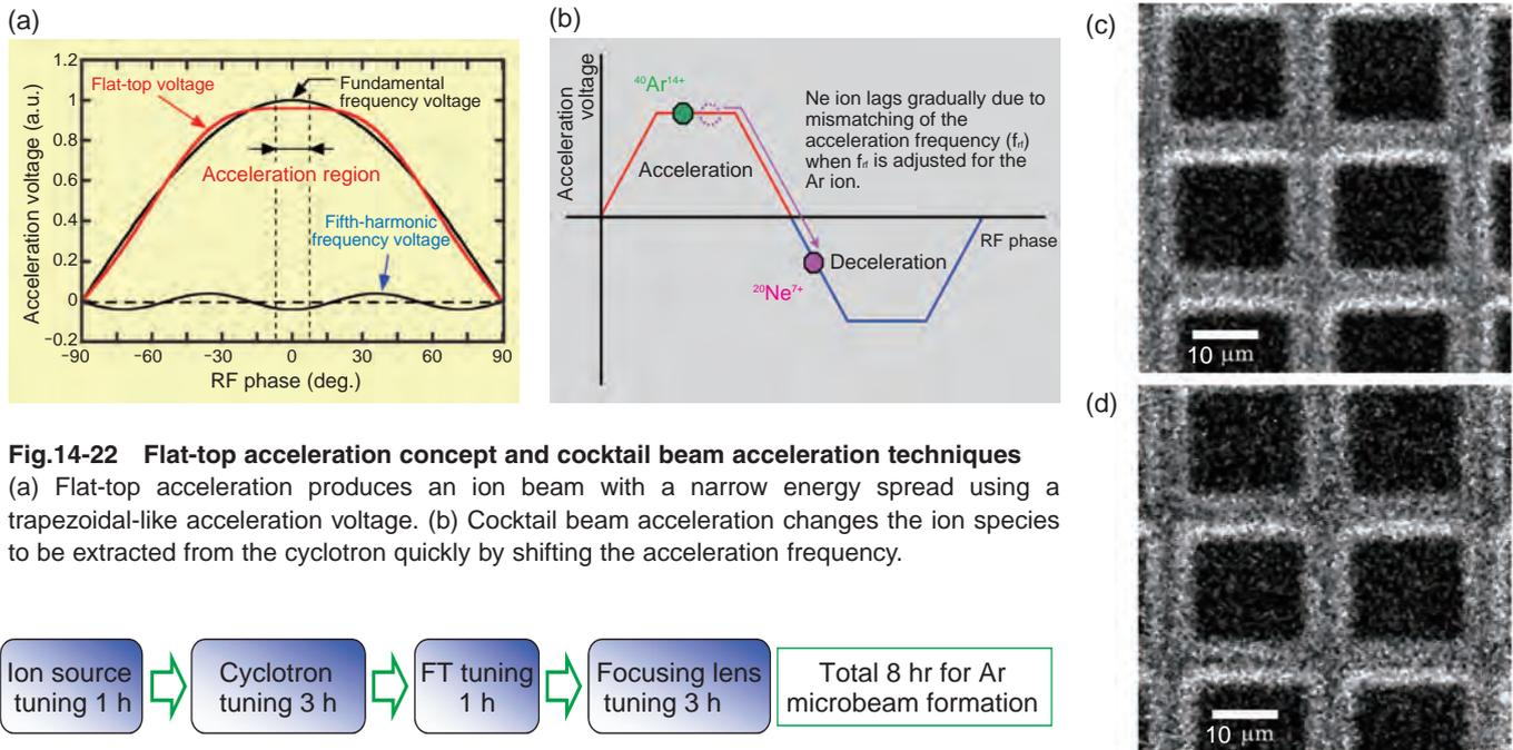
**Fig.14-22 Flat-top acceleration concept and cocktail beam acceleration techniques**
