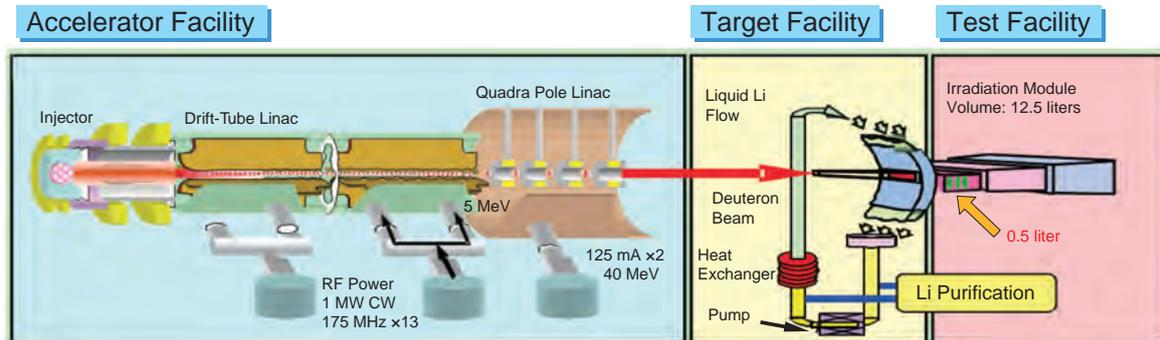
**Fig.3-29 Acceleration-driven type neutron irradiation facility for fusion materials**
