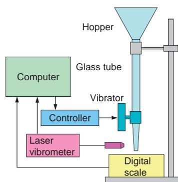
**Fig.1-16 Vibrating tube method schematic diagram**
