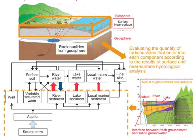
**Fig.2-10 Image of biosphere model development using the information acquired at actual surface and near-surface environments**
