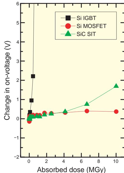
**Fig.4-18 Relationship between absorbed dose and on-voltage**
