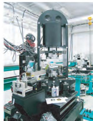
**Fig.4-2 Apparatus for high temperature and pressure X-ray diffraction experiment**
