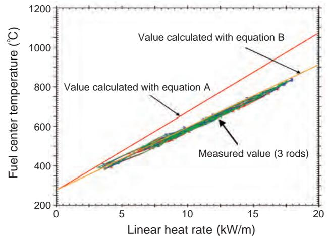
**Fig.6-5 Comparison between measured and calculated fuel temperatures of high burnup MOX fuels**
