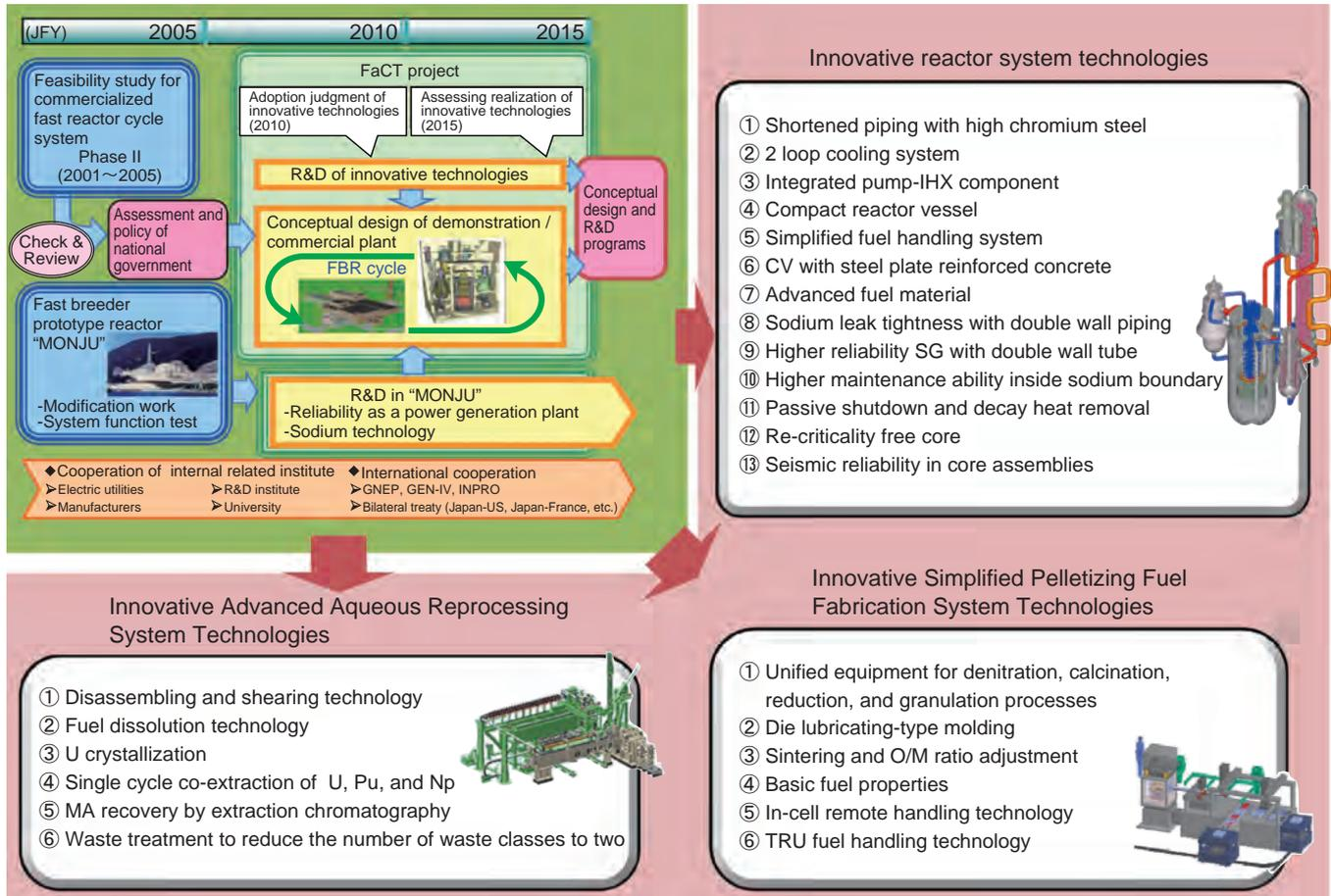
**Fig.1-1 Fast Reactor Cycle Technology Development (FaCT Project)**
