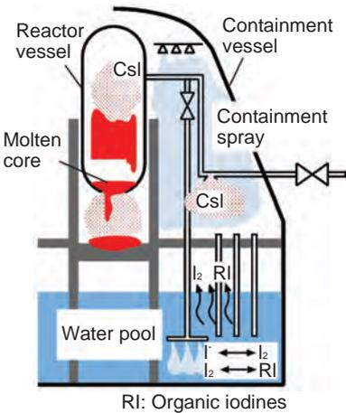
**Fig.6-15 Iodine release during a severe accident**
