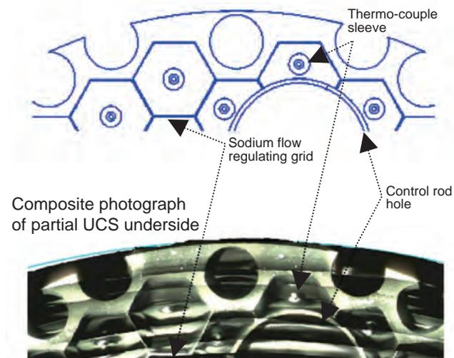
**Fig.14-18 Observation results for the underside of the UCS**
