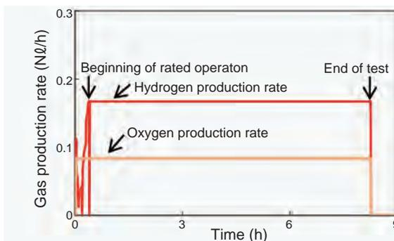
**Fig.14-16 Example of hydrogen production experiment**
