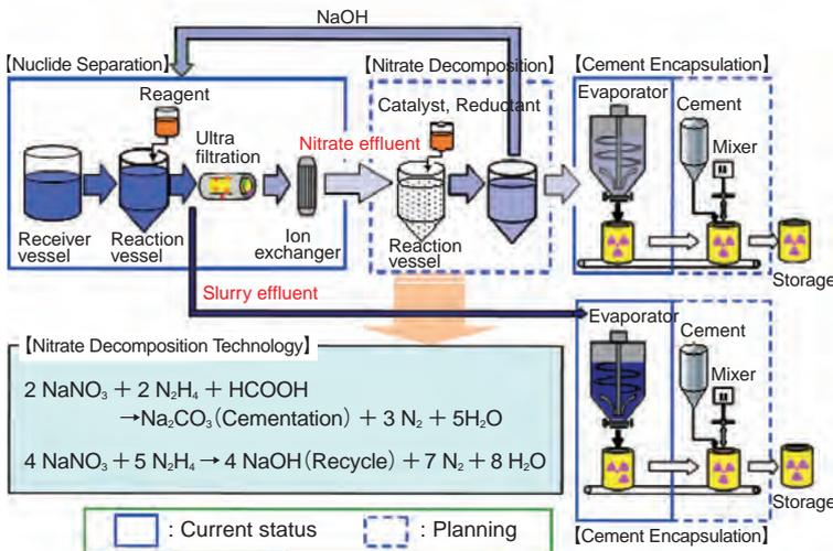
**Fig.10-4 Current status and planning of the effluent treatment**
