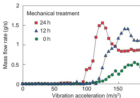
**Fig.1-18 Flowability profiles of ZrO<sub>2</sub> smaller than 45 μm**
