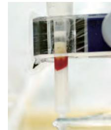
**Fig.11-8 Separation of radioactive nuclides by SPE**
