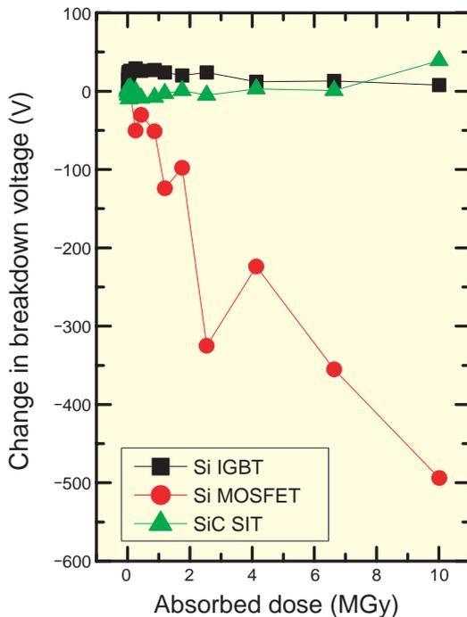
**Fig.4-17 Relationship between absorbed dose and breakdown voltage**
