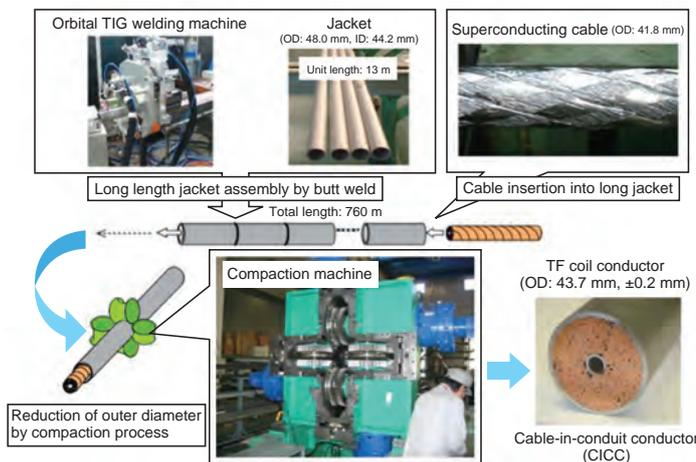
**Fig.3-4 Fabrication process of the TF conductor**
