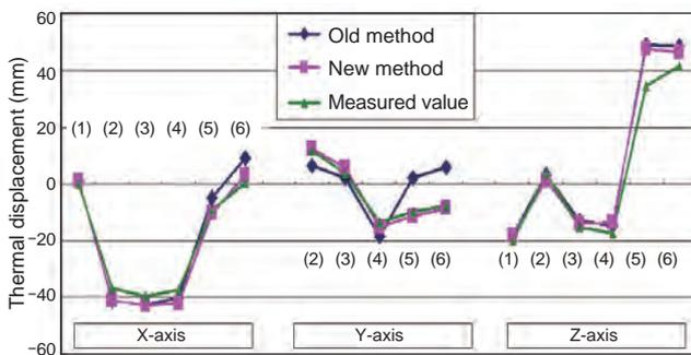
**Fig.14-21 Measurement and analysis of thermal displacement**
