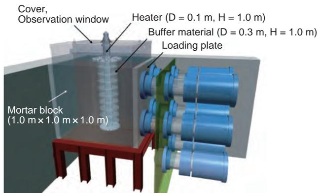
**Fig.2-4 Schematic view of the engineered barrier experiment**
