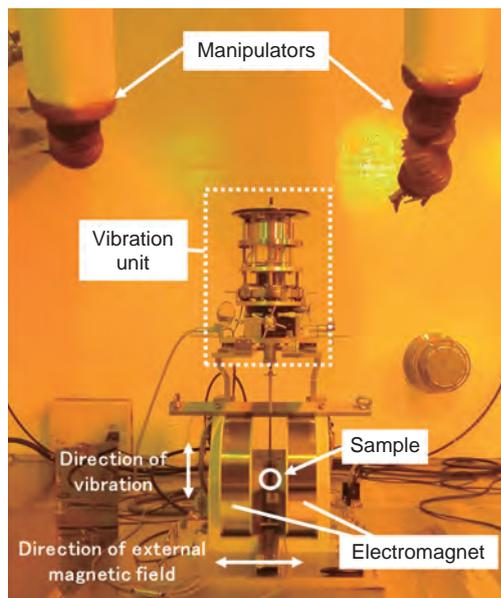
**Fig.1-27 Remote operated VSM in a hot cell**
