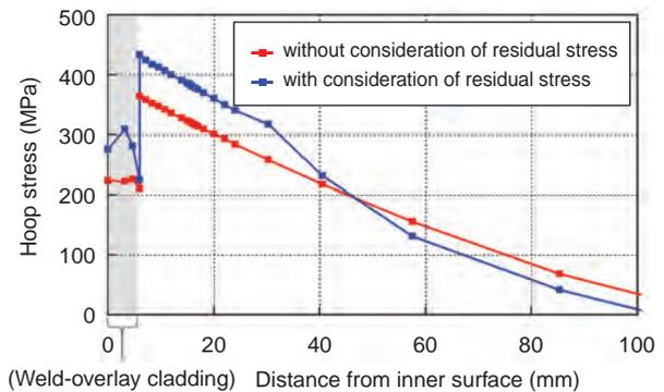
**Fig.6-11 Hoop direction stress with or without consideration of residual stress due to overlay welding during PTS**
