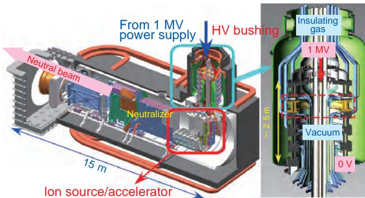
**Fig.3-9 ITER NBI system and high voltage bushing**
