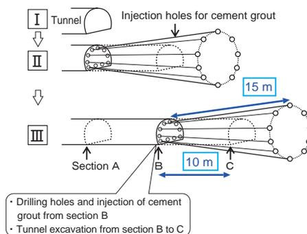
**Fig.14-28 Pre-excavation grouting and tunnel excavation pattern**
