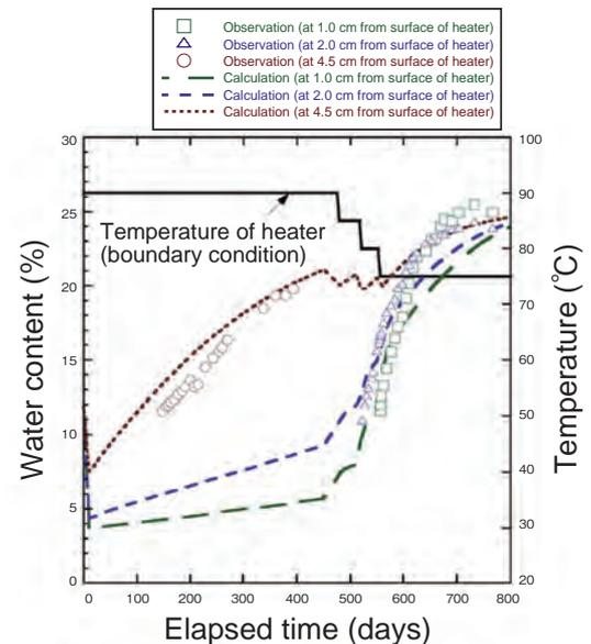
**Fig.2-5 Comparison of calculated and measured water content of the buffer material at the depths indicated as a function of elapsed time**
