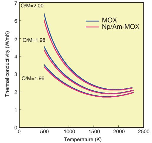
**Fig.1-21 Temperature dependence of thermal conductivity**
