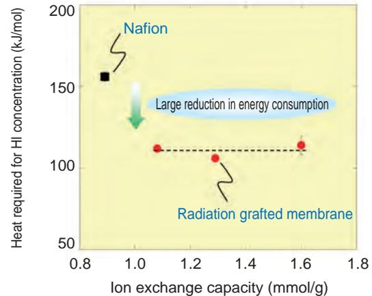
**Fig.9-4 Performance comparison between radiation-grafted membranes and commercially available membranes**
