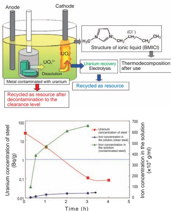
**Fig.14-29 Outline of uranium recovery technique using ionic liquid**
