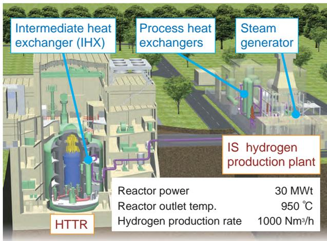
**Fig.9-5 HTTR-IS nuclear hydrogen production system**
