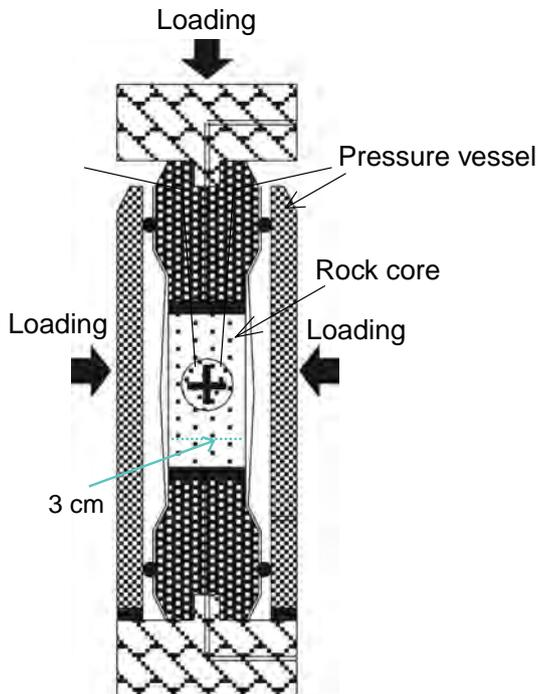
**Fig.2-18 System of laboratory testing**
