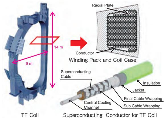
**Fig.3-3 Structure of TF coils and their superconductor**
