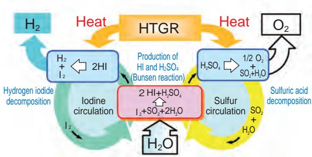
**Fig.9-2 Schematic representation of the IS process**
