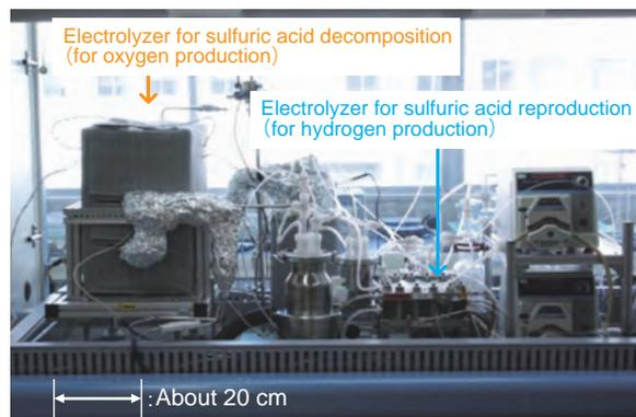
**Fig.14-15 External view of HHLT engineering test apparatus**
