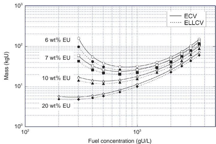
**Fig.6-19 Critical mass data for homogeneous ADU(II)-H<sub>2</sub>O (with water reflector)**
