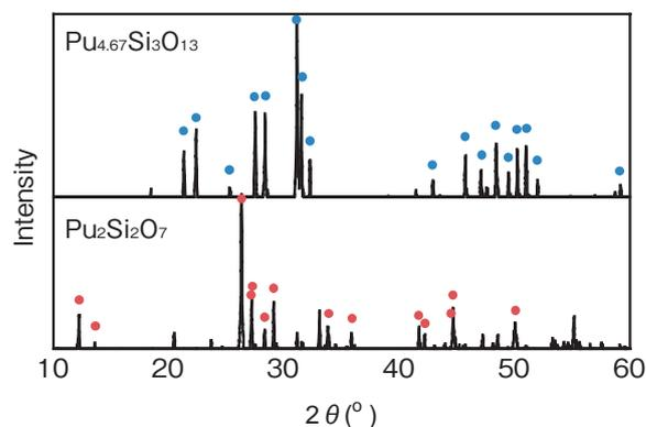
**Fig.1-24 X-ray diffraction patterns of PuO<sub>2</sub>-SiO<sub>2</sub> mixed powders after annealing**
