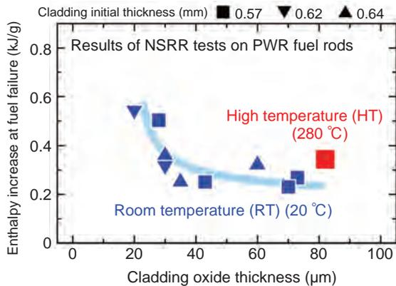
**Fig.6-2 Relation between fuel enthalpy increase at failure and cladding oxide thickness**
