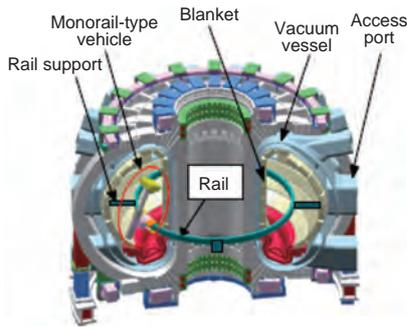
**Fig.3-5 In-vessel remote handling robot for the ITER**
