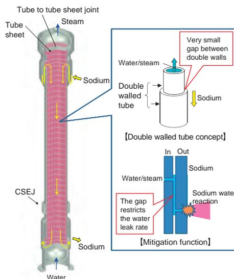
**Fig.1-3 Schematic image of reliable SG**
