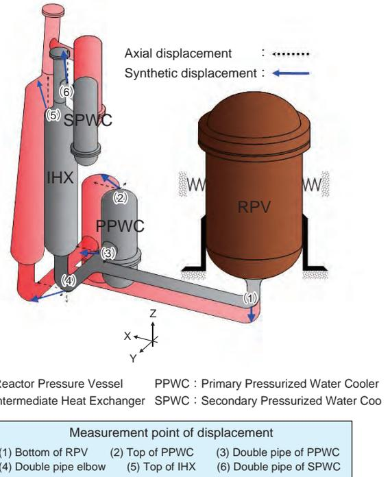
**Fig.14-20 Measured value of displacement behavior**
