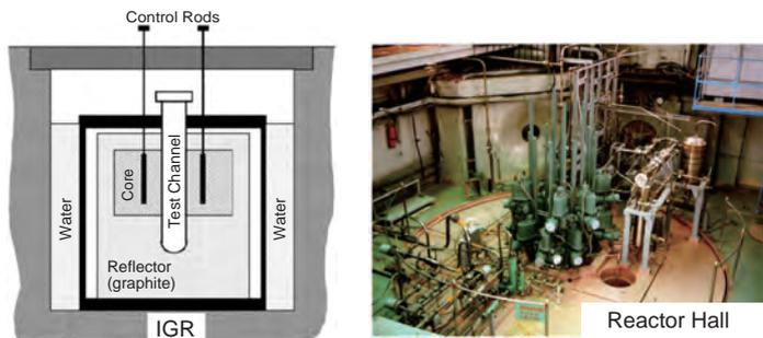
**Fig.1-5 IGR and test channel**
