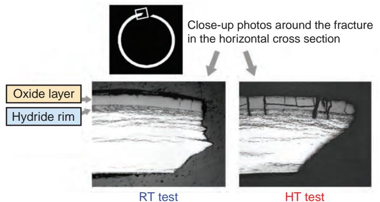
**Fig.6-3 High burnup PWR fuel cladding that failed in the room temperature and high temperature tests at NSRR**
