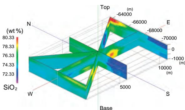
**Fig.2-13 Contoured spatial distribution of SiO<sub>2</sub> concentration in a fence diagram along the red lines in borehole site map (Fig.2-12)**
