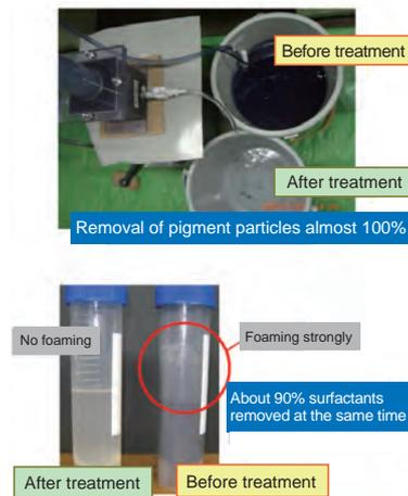
**Fig.8-21 Example of purifying a paint waste solution**
