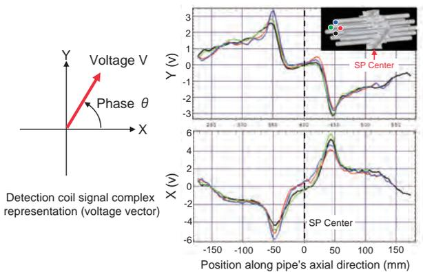
**Fig.1-9 Variation in the SP signal according to various tube positions**
