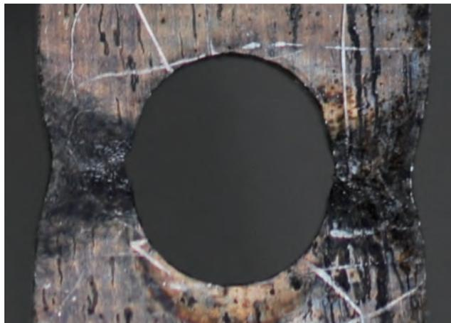
**Fig.8-11 Deformation behavior of an intensely irradiated structure with a discontinuity**
