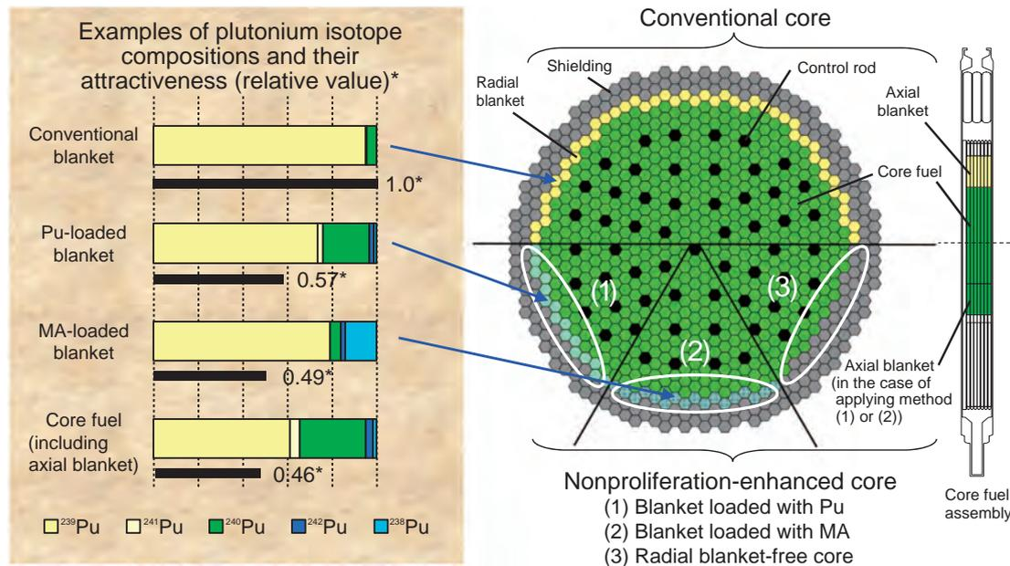
**Fig.1-4 Core design methods to enhance the nonproliferation characteristics of the commercial FBR in terms of a material barrier**
