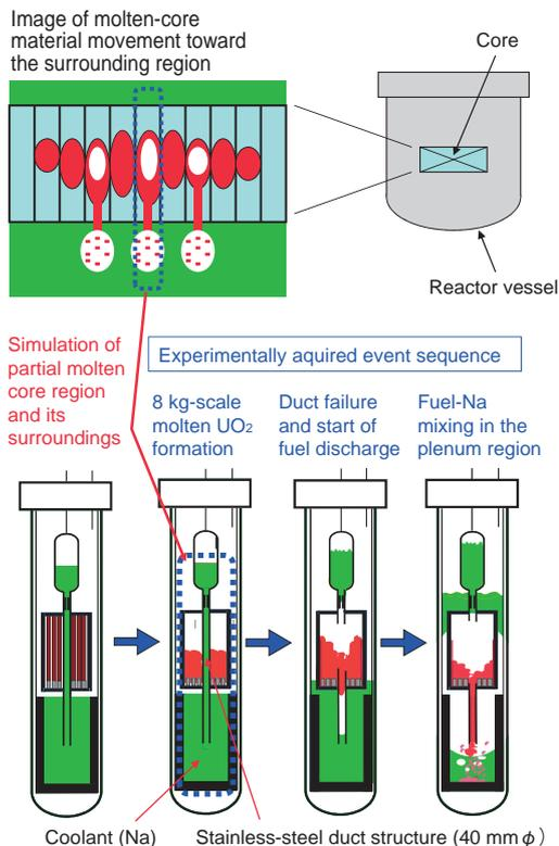
**Fig.1-6 Molten core simulation concept in the experiments**
