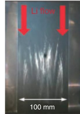
Fig.3-29 Flow appearance of Li target The Li target was formed in the target assembly and flowed stably in the final phase of the performance tests. (The Li target was observed through the observation windows shown in Fig. 3-28).
