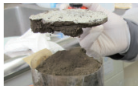
Fig.7-3 Soil solidification technique using polyions
