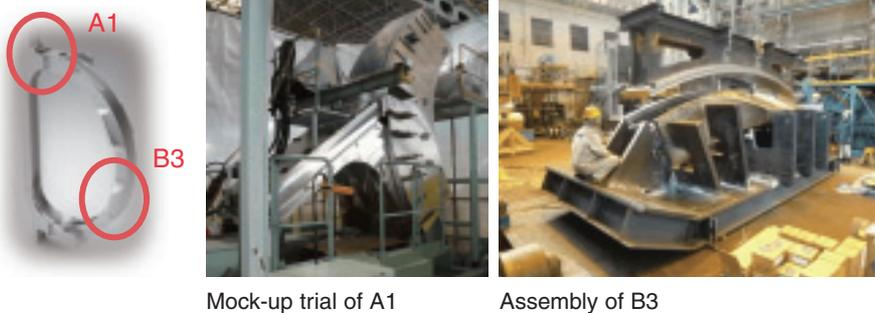
**Fig.3-5 Full-scale segments of coil case**
