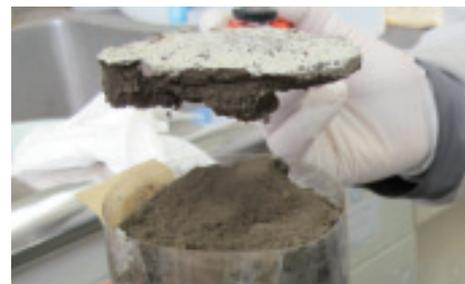
**Fig.7-3 Soil solidification technique using polyions**
