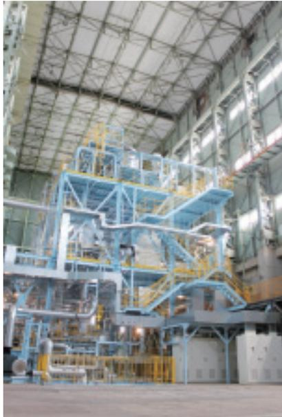
**Fig.12-16** The IFMIF/EVEDA lithium test loop (ELTL)
