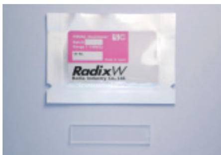
**Fig.12-23** Clear polymethylmethacrylate (PMMA) dosimeter, Radix W
