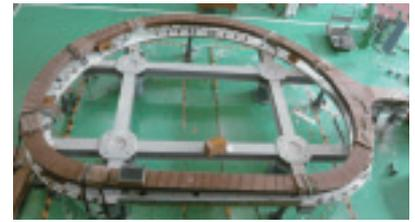
**Fig.3-3 Insulated one-third-scale double pancake (5.1 m × 3.8 m)**
