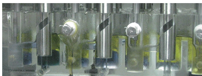
Fig.1-35 The situation of Pu stripping in the partitioning unit
