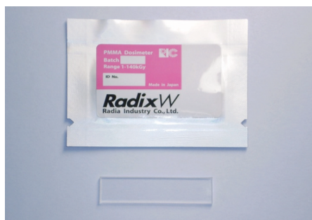
Fig.12-23 Clear polymethylmethacrylate (PMMA) dosimeter, Radix W
