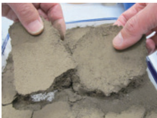
Fig.1-20 Solidification of soil flakes
