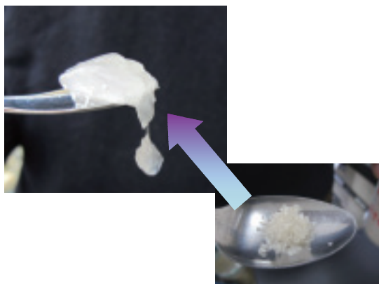
Fig.1-21 Swelling of the poly-ion complex
