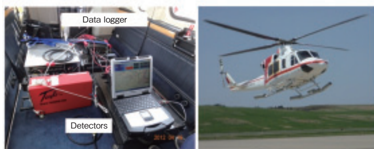
Fig.1-11 Airborne radiation monitoring system
