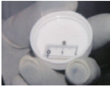
Fig.8-11 (\text{Zr}_{0.58}\text{Pu}_{0.21}\text{Am}_{0.21})\text{N} sintered compact Appearance of high-density sintered compact with a diameter of about 3 mm. Photograph was taken in a glove box.
