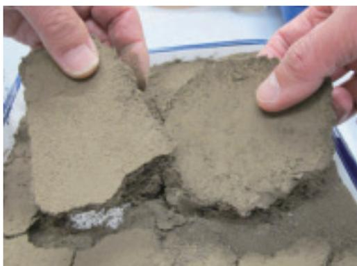
**Fig.1-20 Solidification of soil flakes**
