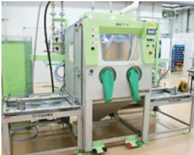
**Fig.13-1 Wet blast decontamination device (manual type)**
