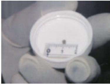
**Fig.8-11**  $(\text{Zr}_{0.58}\text{Pu}_{0.21}\text{Am}_{0.21})\text{N}$  sintered compact
