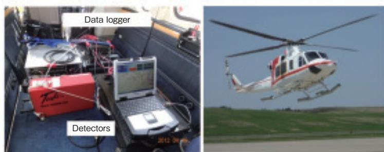
**Fig.1-11 Airborne radiation monitoring system**
