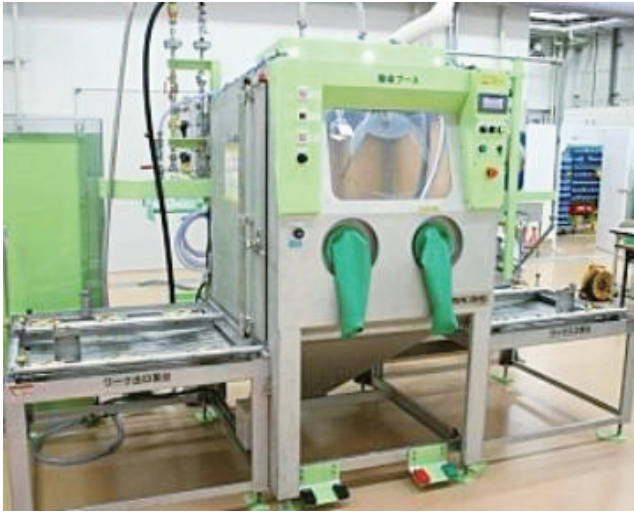
Fig.13-1 Wet blast decontamination device (manual type) The system is composed of a decontamination booth, a blast material sucker, a wastewater treatment system, an exhauster, and an air compressor. Decontamination is to be done by a blast gun in the booth.
