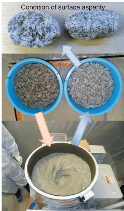
Fig.1-8 Decontamination test by milling method We tested gravel decontamination using a general-purpose barrel finishing machine with 20 kg of gravel, 20 ℓ of water, 150 rounds per min, and 20–60 min of grinding time per batch.
