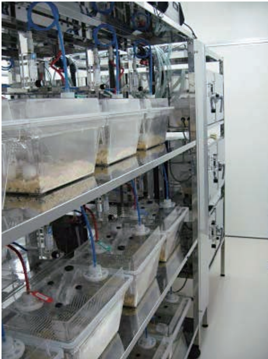
Fig.13-24 Animal test chamber for radon inhalation
