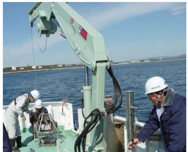
Sampling of seabed soil with a monitoring boat
