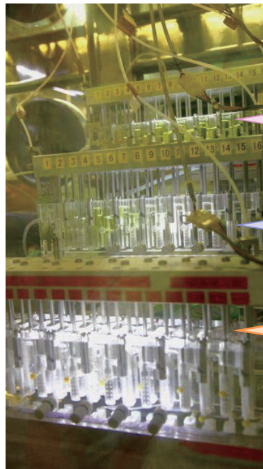
Fig.8-15 Photograph of continuous extraction experiment using mixer-settler extractors for U and Pu extraction
