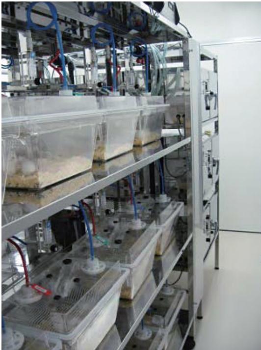
Fig.13-24 Animal test chamber for radon inhalation
