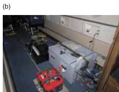
Fig.1-4 Airplane used for the airborne monitoring (a), and the measurement instrument comprising three embedded NaI scintillation detectors (b)
