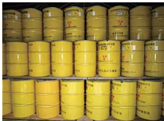
Fig.8-6 Drums for storing sludge-like uranium-bearing waste
