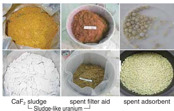
Fig.8-7 Sludge-like uranium and the spent adsorbent
