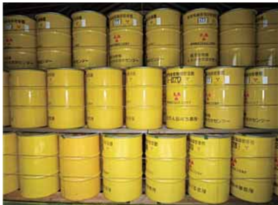
Fig.8-6 Drums for storing sludge-like uranium-bearing waste
