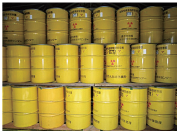
Fig.8-6 Drums for storing sludge-like uranium-bearing waste
