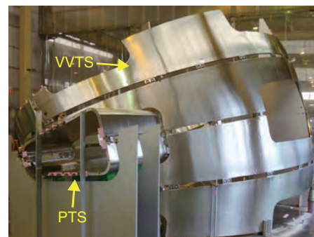
Fig.9-15 Pre-assembly of VVTS Four sets of VVTSs (10°) are assembled to measure dimensions and to adjust the shape of the coupler.
