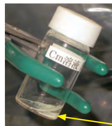
Fig.4-14 The Cm oxalate sample that we prepared
