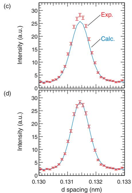
**Fig.5-16 *In situ* neutron diffraction profile at 988 K, 6.3 GPa**
