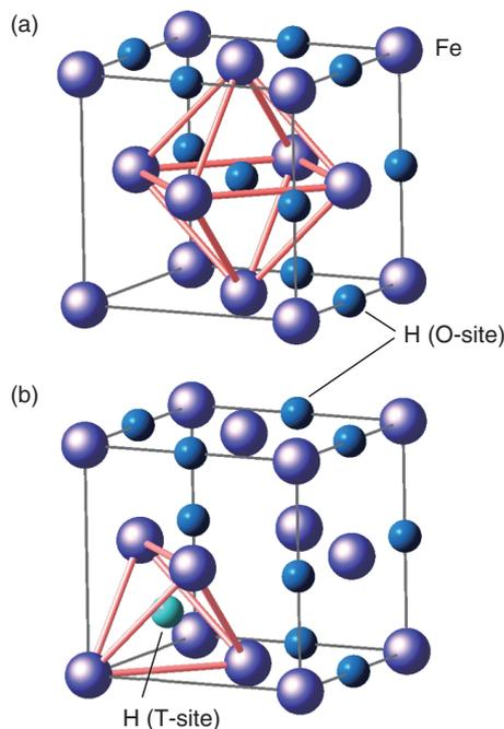
**Fig.5-15 Structural models of  $\text{FeD}_x$  with an fcc metal lattice**
