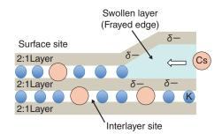
Fig.1-33 A model of radioactive-cesium adsorption into WB
