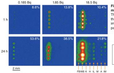
Fig.1-31 Read-out images of IPs with particles of various minerals adsorbing <sup>137</sup>Cs from the solutions
