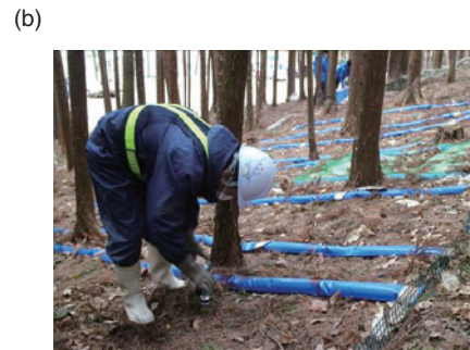
Fig.1-37 (a) Distribution of radioactive Cs on the slope after three months and (b) Appearance of soil-core sampling on the slope The abundance ratios of radioactive Cs on the slope at the upper (1 m), middle (2.5 m), and lower (4 m) positions below the leaf-mold zone is indicated using a bar chart, showing a photo of soil-core sampling at each position.
