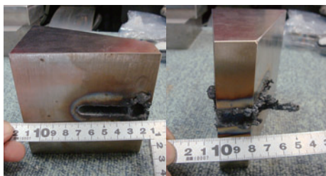
Fig.1-10 Stainless steel after cutting
