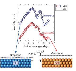
Fig.3-8 Intensity of diffracted positrons for graphene/Co and graphene/Cu and analytical results
