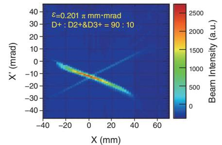
Fig.9-20 Phase-space distribution of extracted beam-ion species
