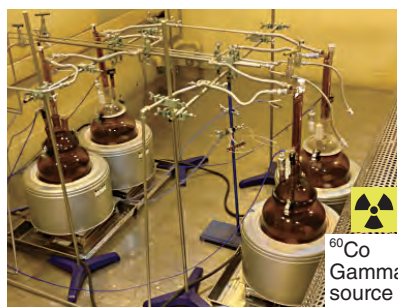
Fig.1-15 The appearance of the test equipment in the gamma-irradiation room and a schematic of the electrochemical-testing cell
