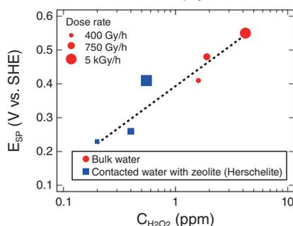
**Fig.1-17** The relationship between the spontaneous potential  $E_{SP}$  of type 316L and hydrogen peroxide concentration  $C_{H_2O_2}$  in the bulk water and the water in contact with zeolites under irradiation
