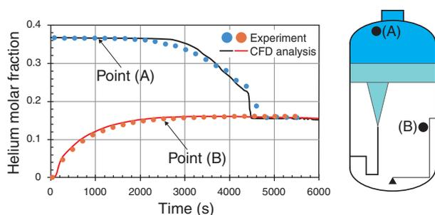
**Fig.2-5 Comparison between the experimental and CFD results for the time history of the helium molar fraction**
