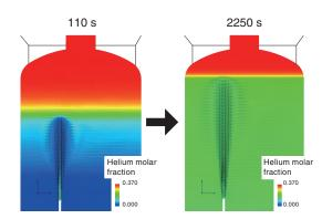
Fig.2-4 Visualization of simulated instantaneous helium molar fraction and velocity vector
