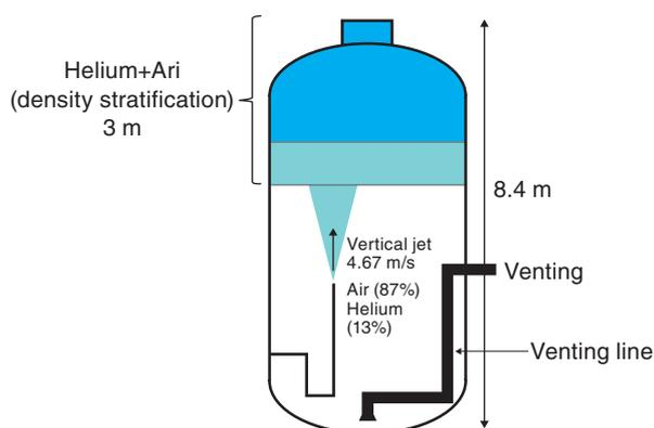
**Fig.2-3 Schematic view of the IBE-3 experimental condition**
